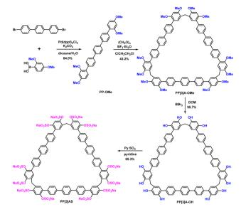
Fig. 2 The synthesis route to pentaphen[3]arene sulfates (PP[3]AS)
