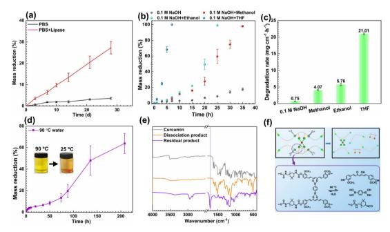
Fig. 6 (a) Mass loss curve of PICB<sub>1.0</sub>PU elastomer in the PBS solution without and with lipase. (b) Mass loss curves and (c) degradation rates of PICB<sub>1.0</sub>PU elastomers in the presence of alkali solutions. (d) Mass loss curve, (e) FT-IR spectra, and (f) schematic illustration of the degradation mechanism of PICB<sub>1.0</sub>PU elastomers in the hot water environment.
