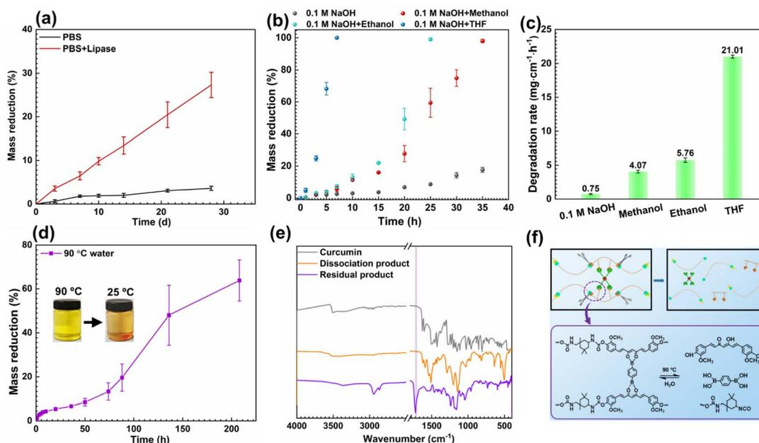
Fig. 6 (a) Mass loss curve of PICB<sub>1,0</sub>PU elastomer in the PBS solution without and with lipase. (b) Mass loss curves and (c) degradation rates of PICB<sub>1,0</sub>PU elastomers in the presence of alkali solutions. (d) Mass loss curve, (e) FT-IR spectra, and (f) schematic illustration of the degradation mechanism of PICB<sub>1,0</sub>PU elastomers in the hot water environment.
