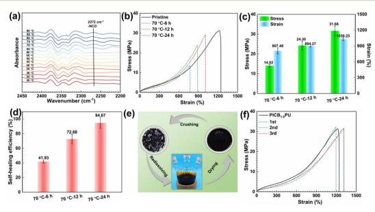
Fig. 4 (a) In situ FT-IR spectra of PICB<sub>1.0</sub>PU elastomers. (b) Stress-strain curves, (c) mechanical properties, and (d) self-healing efficiency of damaged PICB<sub>1.0</sub>PU elastomers after healing for 6 h, 12 h, and 24 h at 70 °C. (e) Schematic illustration of solvent recovery and reprocessing of PICB<sub>1.0</sub>PU elastomers and (f) stress-strain curves for multiple cycles.
