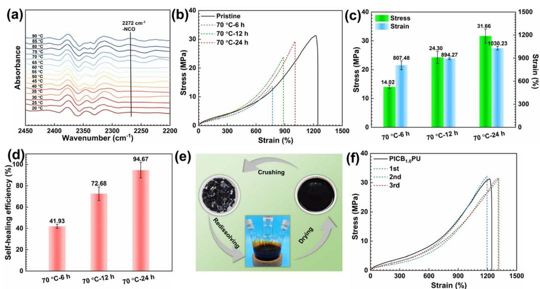
Fig. 4 (a) *In situ* FT-IR spectra of PICB<sub>1,0</sub>PU elastomers. (b) Stress–strain curves, (c) mechanical properties, and (d) self-healing efficiency of damaged PICB<sub>1,0</sub>PU elastomers after healing for 6 h, 12 h, and 24 h at 70 °C. (e) Schematic illustration of solvent recovery and reprocessing of PICB<sub>1,0</sub>PU elastomers and (f) stress–strain curves for multiple cycles.
