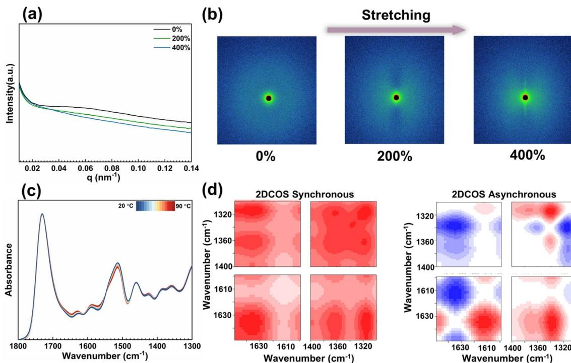
Fig. 2 (a) 1D SAXS profiles at different strains of the PICB<sub>1.0</sub>PU elastomer. (b) 2D SAXS patterns of the PICB<sub>1.0</sub>PU elastomer during stretching. (c) Temperature-variable transmission IR spectra of PICB<sub>1.0</sub>PU elastomer upon heating from 20 to 90 °C (interval: 5 °C). (d) 2D COS synchronous and asynchronous spectra generated from (c). In 2D COS spectra, red color represents positive intensities, while blue color represents negative intensities.
