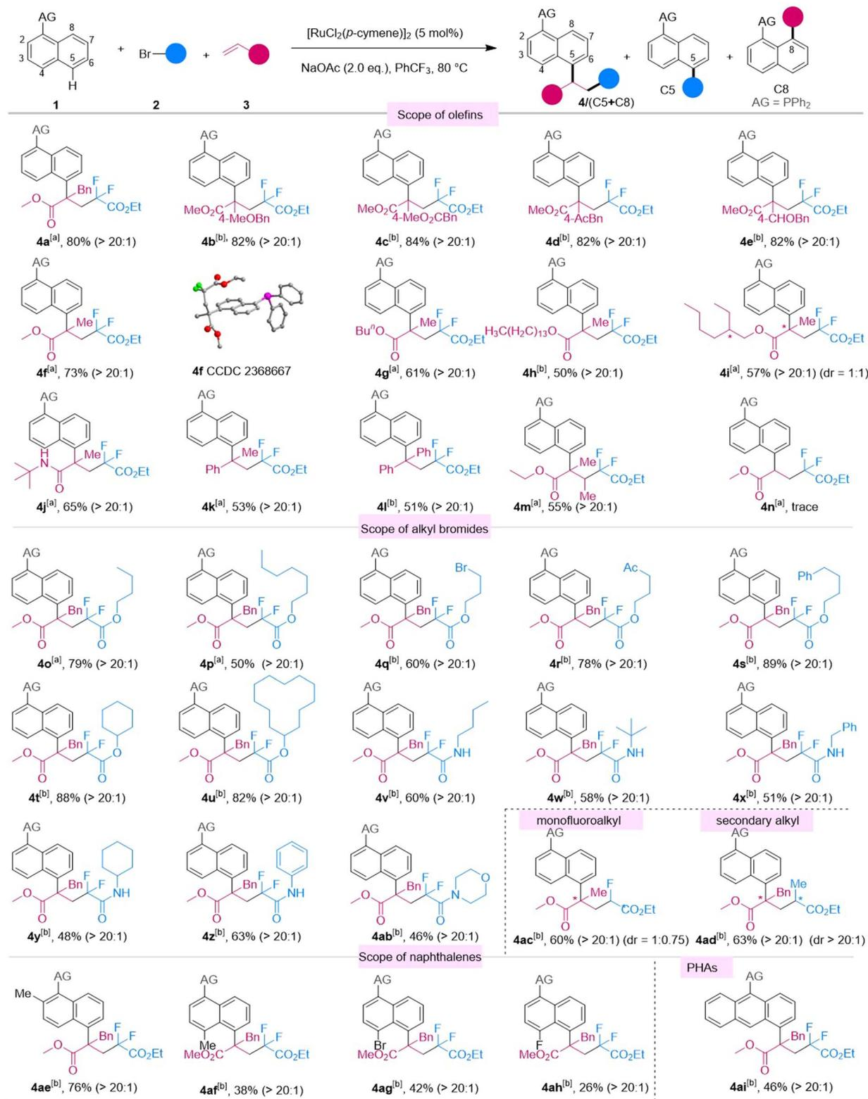
**Scheme 1** Scope of three-component C5-tandem functionalization of naphthalenes with olefins and alkyl bromides. <sup>a</sup>Reaction conditions: 1 (0.10 mmol), 2 (0.30 mmol), 3 (0.30 mmol), 5 mol% [RuCl<sub>2</sub>(*p*-cymene)]<sub>2</sub>, NaOAc (2 equiv.), 1 mL PhCF<sub>3</sub>, in sealed Schlenk tubes, 12 h, 80 °C, under argon; selectivity was determined using <sup>31</sup>P NMR. <sup>b</sup>Oxidized by H<sub>2</sub>O<sub>2</sub>.
