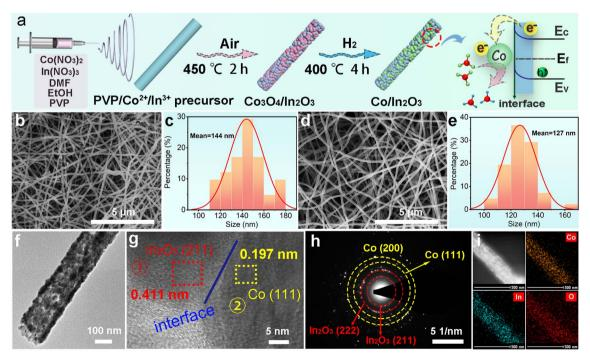
Fig. 1 (a) Synthesis procedure of  $Co/ln_2O_3$ . (b) SEM image and (c) diameter distribution of  $Co_3O_4/ln_2O_3$  nanofibers. (d) SEM image and (e) diameter distribution of  $Co/ln_2O_3$  nanofibers. (f) TEM, (g) HRTEM and (h) SAED images of  $Co/ln_2O_3$ . (i) HAADF-STEM image and EDX element mappings of Co-K, In-L, and O-K.
