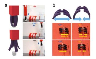
Fig. 12 (a) Ionic bending actuator for bionic gripper and (b) soft locomotive robots. Reproduced with permission.<sup>276</sup> Copyright 2023, Elsevier.
