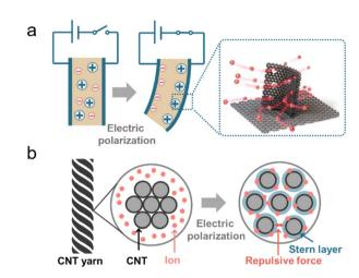
Fig. 9 (a) The mechanism of bending actuators based on a 3D porous graphitic nanoribbon-graphene hierarchical porous structure. Reproduced with permission.<sup>235</sup> Copyright 2020, John Wiley and Sons. (b) The mechanism of a CNT yarn-based ionic actuator. Reproduced with permission.236 Copyright 2024, Elsevier.
