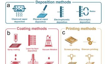
Fig. 4 Fabrication methods of iontronic devices. (a) Deposition methods; (b) coating methods; (c) printing methods.
