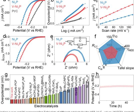
Fig. 3 (a) Polarization curves and (b) corresponding Tafel plots of different catalysts for the HER. (c)  $C_{\rm cl}$  values, (d) ECSA-normalized polarization curves, (e) EIS plots and (f) HER performance radar chart of Ni<sub>2</sub>P and V-Ni<sub>2</sub>P. (g) Overpotential comparison of V-Ni<sub>2</sub>P with reported catalysts. (h) Durability test of V-Ni<sub>2</sub>P.
