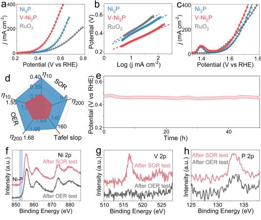
Fig. 4 Polarization curves of the (a) SOR, (b) corresponding Tafel plots and (c) OER of the catalysts. (d) SOR and OER performance radar chart of Ni<sub>2</sub>P and V-Ni<sub>2</sub>P. (e) Durability test of V-Ni<sub>2</sub>P. XPS spectra of (f) Ni 2p, (q) V 2p and (h) P 2p after SOR and OER tests.
