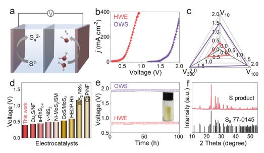
Fig. 5 (a) Schematic illustration of the assembled two-electrode HWE electrolyzer. (b) Polarization curves and durability tests of HWE and OWS systems. Voltage comparison of V-Ni<sub>2</sub>P with (c) HWE and OWS systems at 10, 200 and 300 mA cm<sup>-2</sup>, and (d) recently exploited catalysts. (e) Durability test of V-Ni<sub>2</sub>P for OWS and HWE. Inset: digital image of the S product. (f) XRD pattern of the collected S product.
