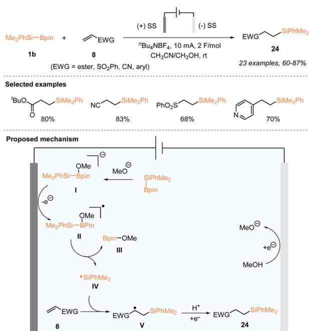
Scheme 8 Electrochemical hydrosilylation of alkenes with  $\text{PhMe}_2\text{Si-Bpin}$ .
