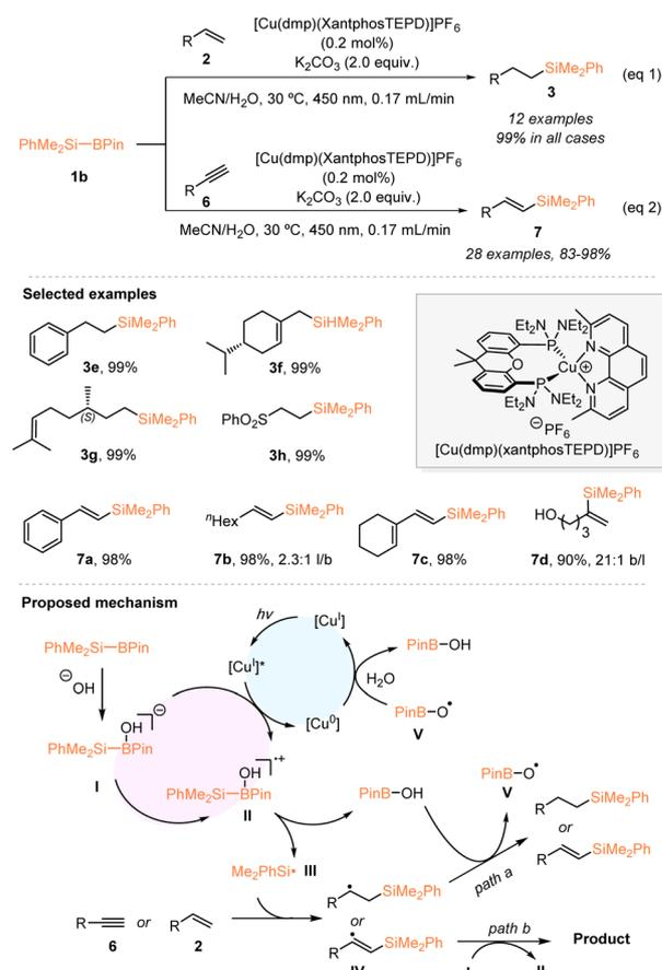
Scheme 2 Copper-photocatalyzed hydrosilylation of alkenes or alkynes with PhMe<sub>2</sub>Si–Bpin.
