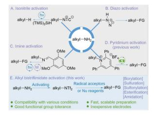
Fig. 1 The strategies of amine activation for deaminative functionalization. (A) Isonitrile activation. (B) Diazo activation. (C) Imine activation. (D) Pyridinium activation. (E) Alkyl bistriflimidate activation.
