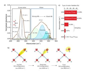
Fig. 3 (a) Illustrative fitting of FTIR spectra within the 2600–3800 cm $^{-1}$  range for C7SeO $_{10}$ -H $_1$  at 25 °C. (b) Schematic depiction of three distinct types of OH configurations in the water network. (c) Percentage distribution of ice-like, distorted, and free OH stretching components derived from the fitting of FTIR spectra for C7SeO $_{10}$ -H $_1$ .
