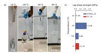
Fig. 5 Application of C7SeO $_{10}$ -H $_1$  materials as adhesive materials at extremely low temperatures. (a) Digital image of lap shear tests performed at -40 °C. Cartoon representation of the adhesion procedure. (b) Macroscopic adhesive behaviour of C7SeO $_{10}$ -H $_1$  materials on a 304 stainless steel surface at various low temperatures. Water was used in these pictures. (c) Lap shear strengths of C7SeO $_{10}$ -H $_1$  and its control C7 $_{10}$ -H $_1$ .
