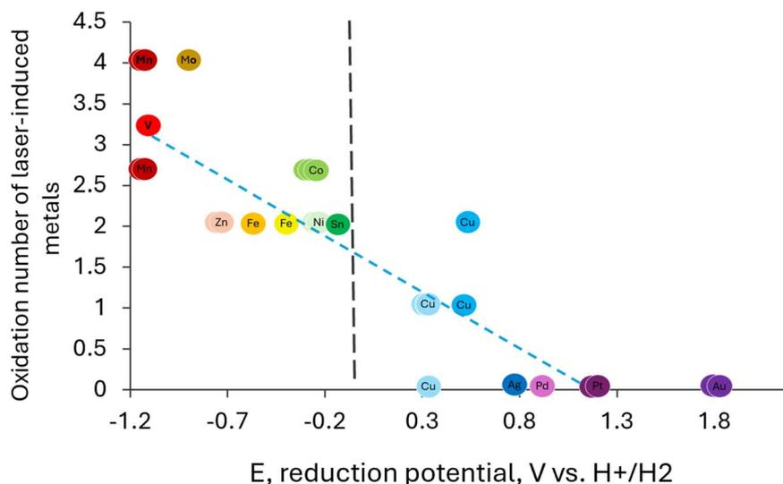
Fig. 1 The oxidation state of laser-induced metals vs. the reduction potential, referring to  $\text{M}^{x+} + x\text{e}^- \rightarrow \text{M}(\text{s})$ . Each color represents a different element. The black line represents the potential of carbon monoxide oxidation. The dashed blue line represents the linear trend. The data and references are presented in Table 1.
