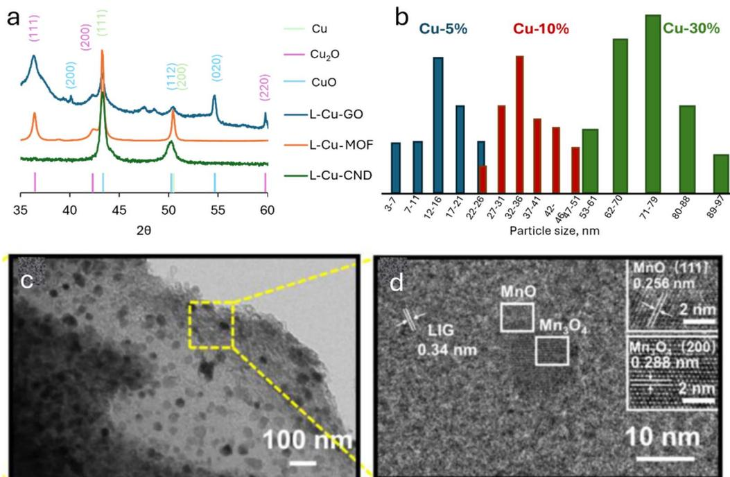
Fig. 2 M-LIG reveals unconventional phenomena. (a) XRD spectra exhibit different copper phases formed from  $\text{Cu}^{2+}$  ions with varying carbon precursors. (b) Particle size distributions formed from three concentrations of  $\text{Cu}^{2+}$  ions lasered under the same conditions. (c) TEM image, (d) HRTEM image and of  $\text{MnO}_x$ @LIG showcasing two manganese-oxide phases in the same particle (taken from ref. 5).
