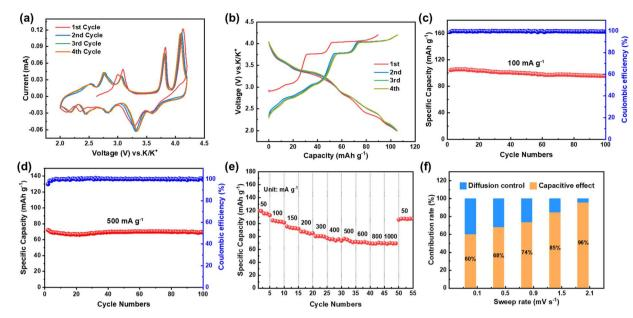
Fig. 3 Buckled-layer  $K_{1.39}Mn_3O_6$  cathode, (a) CV profiles at a scan rate of 0.1 mV s<sup>-1</sup>. (b) Galvanostatic charge-discharge profiles in 1st, 2nd, 3rd and 4th cycles. (c) Cycle performances at a current density of 100 mA g<sup>-1</sup> for 100 cycles. (d) Cycle performances at a current density of 500 mA g<sup>-1</sup> for 100 cycles. (e) Rate capability. (f) Normalized capacitive-controlled capacities and diffusion-controlled capacities at different scan rates.
