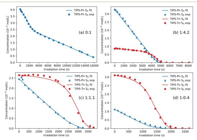
Fig. 6 Fit to the photodegradation of blend TIPS-Tn: TIPS-Pn NPs with mass ratio (a) 0:1, (b) 1:4.2, (c) 1:1.1, and (d) 1:0.4, with the addition of SET and TET from TIPS-Tn to TIPS-Pn. Fits to additional blend ratios are given in the ESI (Fig. S27).† Note that different time axes are used due to the various time scales for photodegradation.
