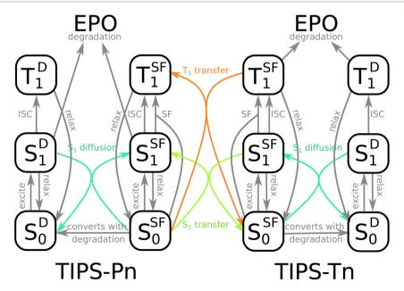
Fig. 5 Model used to fit the photodegradation of TIPS-Tn:TIPS-Pn blend NPs. Processes in gray have known rate constants, taken from the neat systems. Only the processes in color are fit to the blend photodegradation data.
