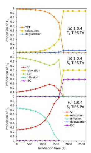
Fig. 8 Change in relative importance of different processes for 1: 0.4 TIPS-Pn: TIPS-Tn NPs over time as the NP degrades, for (a) TIPS-Tn  $T_1$ . (b) TIPS-Tn  $S_1$ , and (c) TIPS-Pn  $S_1$ . Note that proportions of relaxation, degradation, and ISC are coincident (too small to resolve) in (c).
