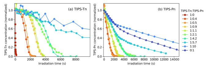
Fig. 3 Photodegradation of TIPS-Tn: TIPS-Pn NPs at various mass ratios: concentration of (a) TIPS-Tn component and (b) TIPS-Pn component vs. irradiation. Concentrations are normalized to the initial data point.
