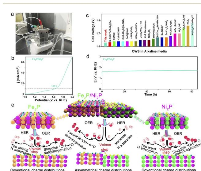
Fig. 8 (a) The AEMWE device. (b) Polarization curves of AEM water electrolyzer with Fe<sub>2</sub>P/Ni<sub>2</sub>P. (c) Comparison of Fe<sub>2</sub>P/Ni<sub>2</sub>P with reported bifunctional electrocatalysts at 10 mA cm<sup>−2</sup>. (d) Stability of Fe<sub>2</sub>P/Ni<sub>2</sub>P//Fe<sub>2</sub>P/Ni<sub>2</sub>P at 10 mA cm<sup>−2</sup> in AEMWE. (e) Schematic illustration of OER and HER mechanisms for Fe<sub>2</sub>P/Ni<sub>2</sub>P bifunctional electrocatalyst.
