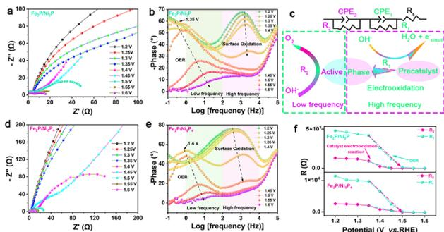
Fig. 6 (a and d) *Operando* Nyquist plots, (b and e) Bode-phase plots of  $\text{Fe}_2\text{P}/\text{Ni}_2\text{P}$  and  $\text{Fe}_2\text{P}/\text{Ni}_5\text{P}_4$ . (c) Electrical equivalent circuit model used for analyzing the interfacial charge transfer. (f) Correlation of the equivalent resistances ( $R_1$  and  $R_2$ ) and potentials for  $\text{Fe}_2\text{P}/\text{Ni}_2\text{P}$  and  $\text{Fe}_2\text{P}/\text{Ni}_5\text{P}_4$ .
