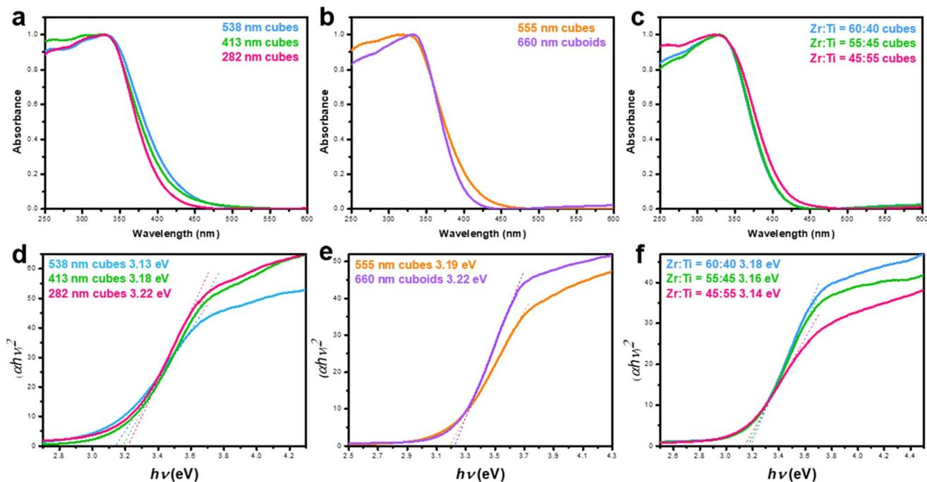
Fig. 7 UV-vis diffuse reflectance spectra of (a) size-tunable  $\text{PbZr}_{0.7}\text{Ti}_{0.3}\text{O}_3$  cubes, (b) 555 nm  $\text{PbZr}_{0.7}\text{Ti}_{0.3}\text{O}_3$  cubes and 660 nm  $\text{PbZr}_{0.7}\text{Ti}_{0.3}\text{O}_3$  cuboids, and (c)  $\text{PbZr}_x\text{Ti}_{1-x}\text{O}_3$  with different Zr : Ti atomic percentages. (d–f) Their corresponding Tauc plots.
