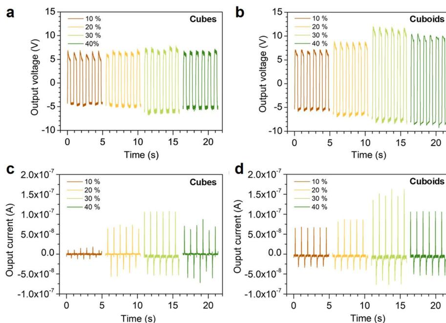
Fig. 9 Electrical output performance characterization of the PENG. (a and b) Open-circuit voltages of  $\text{PbZr}_{0.7}\text{Ti}_{0.3}\text{O}_3$  cubes and cuboids with varying weight percentages. (c and d) Short-circuit currents of these  $\text{PbZr}_{0.7}\text{Ti}_{0.3}\text{O}_3$  cubes and cuboids.
