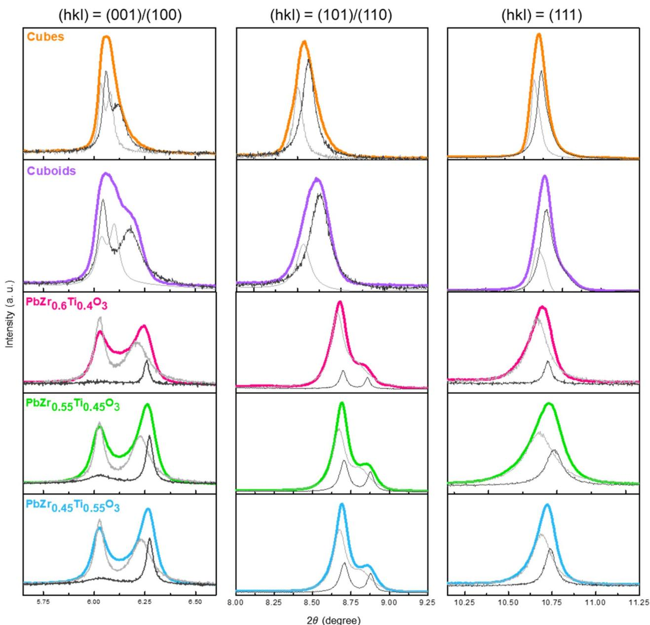
Fig. 3 Expanded (001)/(100), (101)/(110), and (111) synchrotron XRD peaks of  $\text{PbZr}_{0.7}\text{Ti}_{0.3}\text{O}_3$  cubes and cuboids, and  $\text{PbZr}_{0.6}\text{Ti}_{0.4}\text{O}_3$ ,  $\text{PbZr}_{0.55}\text{Ti}_{0.45}\text{O}_3$ , and  $\text{PbZr}_{0.45}\text{Ti}_{0.55}\text{O}_3$  cubes. The gray lines are outcomes of the two-phase simulation from the Rietveld refinement process.
