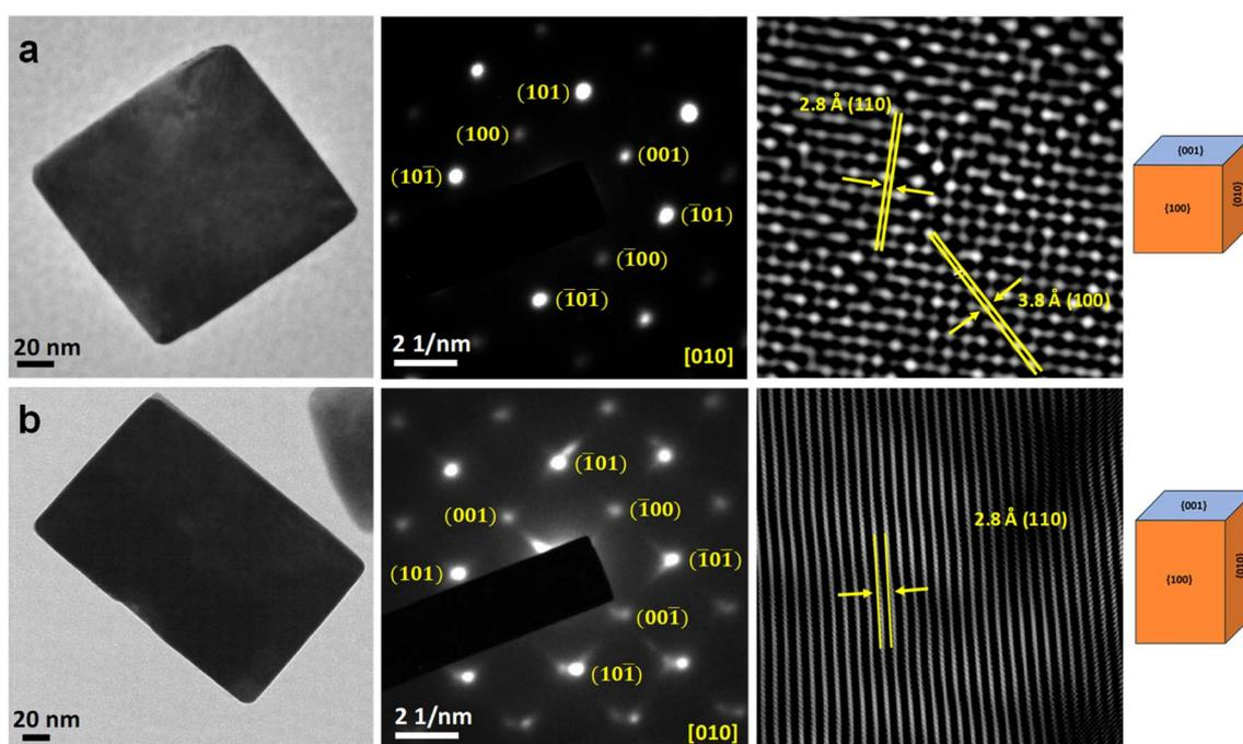
Fig. 4 TEM images, SAED patterns, and FFT-derived lattice point images of (a) a  $\text{PbZr}_{0.7}\text{Ti}_{0.3}\text{O}_3$  cube and (b) a  $\text{PbZr}_{0.7}\text{Ti}_{0.3}\text{O}_3$  cuboid. The models show their exposed faces.
