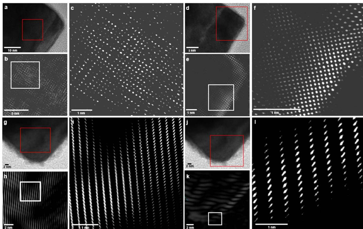
Fig. 5 (a, d, g and j) HR-TEM image of a portion of (a and d) a  $\text{PbZr}_{0.7}\text{Ti}_{0.3}\text{O}_3$  cube and (g and j) a cuboid. (b, e, h and k) The corresponding FFT-derived lattice point images of the red square areas. (c, f, i and l) Enlarged images of the white square areas.
