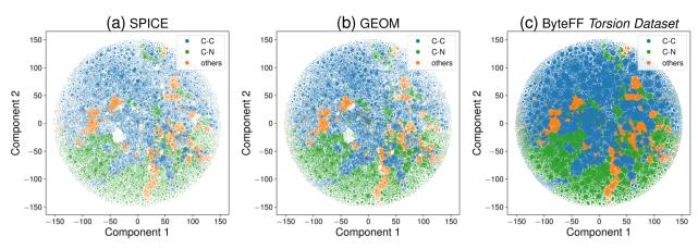
Fig. 2 t-SNE analysis of different datasets, (a) SPICE, (b) GEOM and (c) ByteFF torsion dataset. The Morgan-based torsional fingerprint analysis results are illustrated using the t-SNE algorithm. Every scatter dot corresponds to a torsion profile being analyzed in the corresponding dataset, which is colored by the element types of the two center atoms in the torsion.
