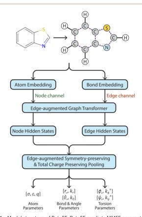
Fig. 1 Model structure of ByteFF. ByteFF predicts MMFF parameters in three steps. First, atom and bond features are extracted from the molecular graph and then projected into embeddings. Then, an edge-augmented graph transformer (EGT)<sup>47</sup> is used to synergize the edge embeddings with the node-based attention mechanism. Lastly, the output module derives force field parameters while preserving the molecular symmetry and total charge.
