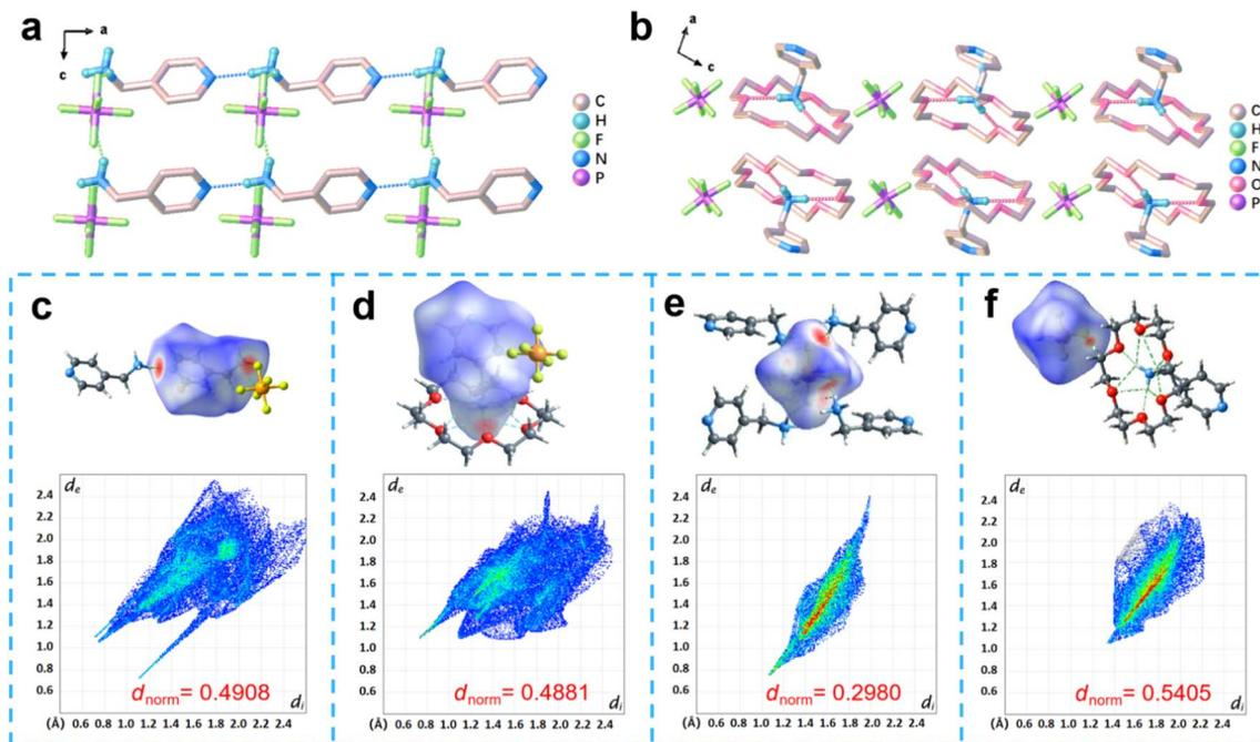
Fig. 1 (a and b) Packing structure of PP-1 (a) and PCP-1 (b) viewed along the crystallographic *b*-axis at 303 K. Pink and blue dashed lines indicate hydrogen bonds, with some hydrogen atoms omitted for clarity. (c and d) Hirshfeld  $d_{\text{norm}}$  surfaces and associated 2D fingerprint plots of the 4-PDMA cations in PP-1 (c) and PCP-1 (d). (e and f) Hirshfeld  $d_{\text{norm}}$  surfaces and associated 2D fingerprint plots of the  $\text{PF}_6^-$  anions in PP-1 (e) and PCP-1 (f).
