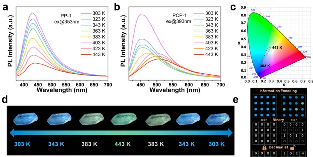
Fig. 4 (a) Temperature-dependent PL spectra ( $\lambda_{ex} = 353$  nm) of PP-1. (b) Temperature-dependent PL spectra ( $\lambda_{ex} = 393$  nm) of PCP-1. (c) Temperature-dependent CIE chromaticity coordinates of PCP-1. (d) Temperature-dependent luminescent colour of the PCP-1 crystals. (e) Schematic of the information encryption and decryption process based on the temperature-dependent PL responses of PP-1 and PCP-1.
