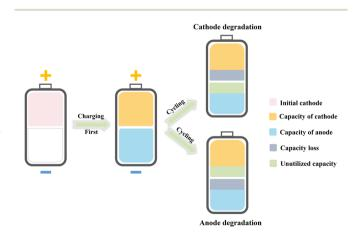
Fig. 2 Illustration of the performance of anode-free metal batteries dictated by capacity decay of either electrode.
