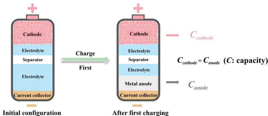
Fig. 1 The anode-free metal battery configuration and the relationship between the theoretical capacities of the cathode and anode.
