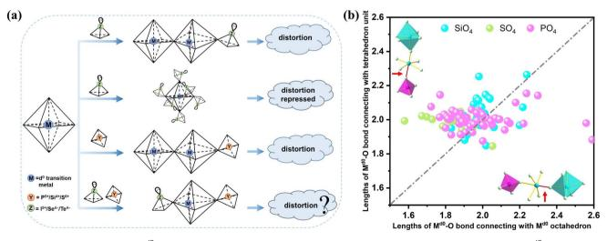
Fig. 1 (a) Schematic diagram of  $[M^{d0}O_6]$  octahedral distortion induced by different connections. (b) Length distribution of  $M^{d0}$ –O bonds in the  $[M^{dO}O_6]$  octahedron connected to other  $[M^{dO}O_6]$  octahedra and tetrahedral units simultaneously in phosphates, sulfates, and silicates containing Md0
