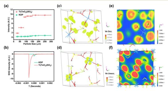
Fig. 3 (a) SHG intensity versus particle size under laser irradiation at 1064 nm with KDP as the reference; (b) oscilloscope traces of the SHG signals (at the sample size range of 200-300 µm); SHG-weighted density map of (c) occupied and (d) unoccupied states in the virtual electron process; calculated electron-density difference of (e) Ti(TeO<sub>3</sub>)(SO<sub>4</sub>) (100) and (f) TiTe<sub>3</sub>O<sub>8</sub> (100).
