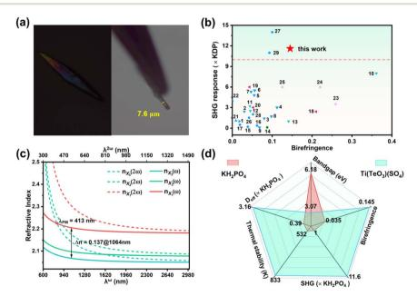
Fig. 4 (a) The original interference color under orthogonal polarized light and thickness of the selected crystal plate of Ti(TeO<sub>3</sub>)(SO<sub>4</sub>); (b) SHG responses and birefringence of some reported sulfates (the numbers insides correspond to the serial numbers of the sulfates listed in Table S7†); (c) the calculated refractive index dispersion curves; (d) properties comparison of Ti(TeO<sub>3</sub>)(SO<sub>4</sub>) with the commercial KH<sub>2</sub>PO<sub>4</sub>.
