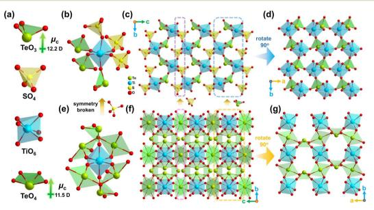
Fig. 2 Structural diagram of  $Ti(TeO_3)(SO_4)$  and  $TiTe_3O_8$ . (a) The anionic groups;  $Ti(TeO_3)(SO_4)$  structure: (b) the  $Ti(TeO_3)_3(SO_4)_3$  unit, (c) the structure viewed along the [100] direction, (d) the [( $TiO_3O_{3/2}$ )( $TeO_3$ )] layer viewed along the [001] direction;  $TiTe_3O_8$  structure: (e) the coordination environment of [ $TiO_6$ ], (f) the structure viewed along the [100] direction, (g) the [( $TiO_2O_4$ )( $TeO_4$ )] layer viewed along the [001] direction.
