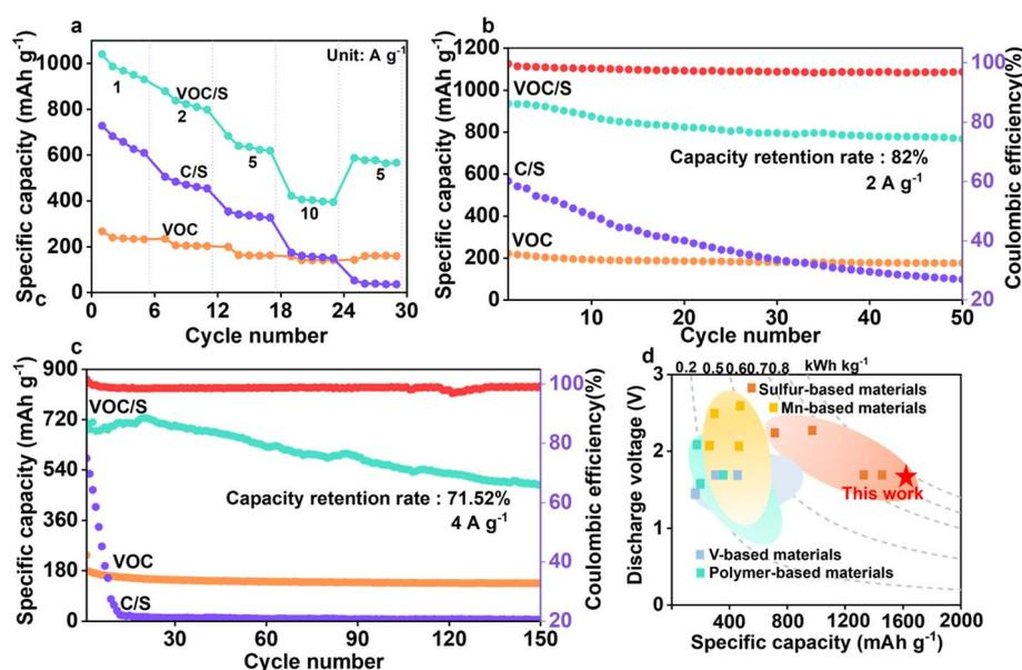
Fig. 4 Electrochemical performance of the VOC/S cathode. (a) Rate performance. Cycle performance at a current density of (b) 2  $\text{A g}^{-1}$  and (c) 4  $\text{A g}^{-1}$ . (d) Electrochemical performances of our work compared with those of previously reported aqueous Zn-ion batteries.
