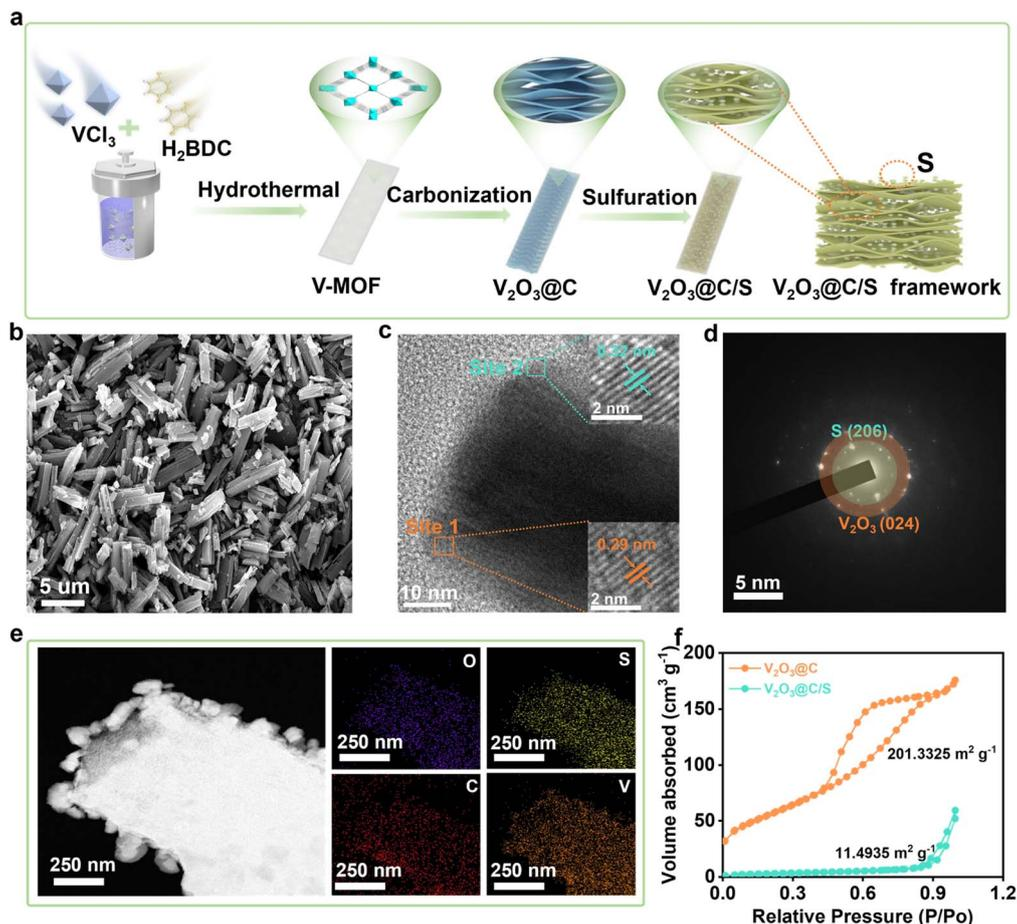
Fig. 1 Structural and compositional characterization of the as-prepared  $V_2O_3@C/S$  precursor. (a) Schematic illustration of the synthesis procedure for the  $V_2O_3@C/S$  composite. (b) SEM images of  $V_2O_3@C/S$ . (c) TEM images of  $V_2O_3@C/S$ . (d) SAED pattern of  $V_2O_3@C/S$ . (e) SEM image of  $V_2O_3@C/S$  and corresponding elemental mappings. (f) Nitrogen adsorption-desorption isotherms of different samples.
