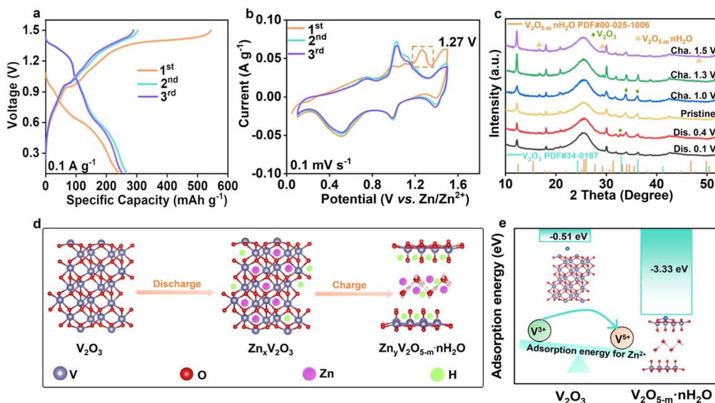
Fig. 2 *In situ* electrochemical reconstruction of the phase of vanadium oxides. (a) Galvanostatic charge/discharge curves of VOC at a current density of  $0.1 \text{ A g}^{-1}$ . (b) CV curves of VOC at  $0.1 \text{ mV s}^{-1}$ . (c) XRD patterns of the VOC cathode at different states. (d) Schematic illustration of the oxidation of  $V_2O_3$  during the first cycle. (e) Adsorption energies of  $V_2O_3$  and  $V_2O_{5-m} \cdot nH_2O$  towards zinc ions.
