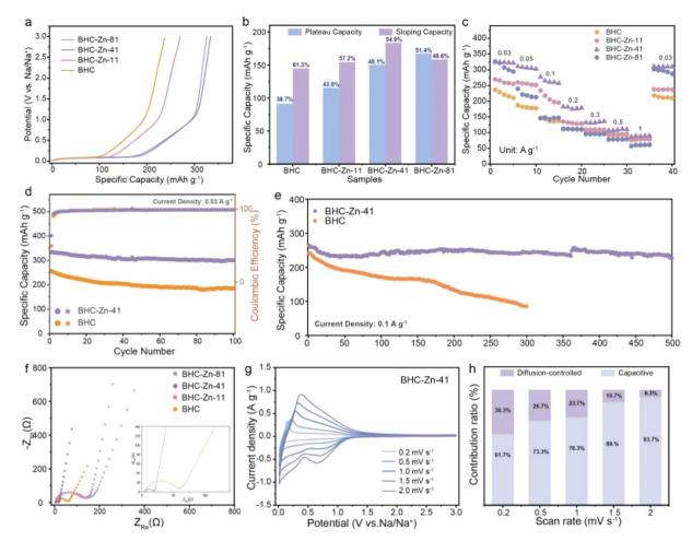
Fig. 3 (a) Galvanostatic charge profiles of all four samples at  $0.03 \text{ A g}^{-1}$ . (b) The percentage of capacity contribution of all four samples. (c) Rate performance of all four samples. Cycle performance of BHC and BHC-Zn-41 at (d) 0.03 A  $g^{-1}$  and (e) 0.1 A  $g^{-1}$ . (f) Nyquist curves of all four samples. (g) CV curves of BHC-Zn-41 at various scan rates. (h) Comparison of contribution ratios of capacitive process and diffusion-controlled at various scan rates
