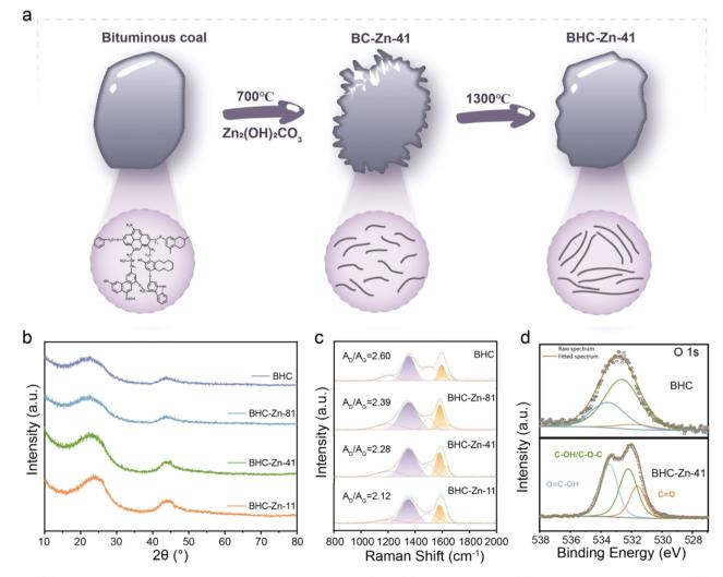
Fig. 1 (a) Schematic representation of the preparation process for BHC-Zn; (b) XRD patterns and (c) Raman spectra of all samples; (d) highresolution O 1s XPS spectra of BHC and BHC-Zn-41.
