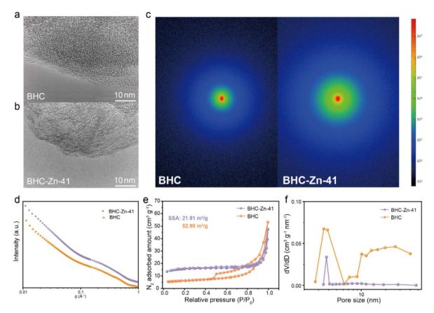
Fig. 2 HRETM images of (a) BHC and (b) BHC-Zn-41; (c and d) SAXS patterns of BHC and BHC-Zn-41; (e) N<sub>2</sub> adsorption/desorption isotherms and (f) pore size distribution of BHC and BHC-Zn-41.
