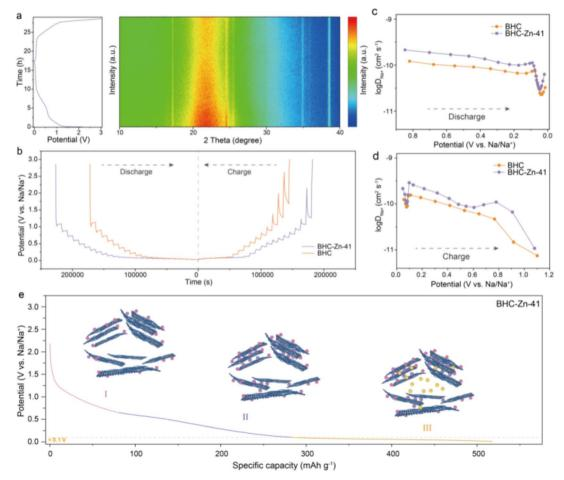
Fig. 4 (a) In situ XRD spectra of BHC-Zn-41 during the first discharge-charge process at  $0.03 \, \text{A g}^{-1}$ . (b) GITT potential profiles and (c and d) the calculated Na<sup>+</sup> diffusion coefficients during the charge/discharge process. (e) Illustration of the sodium storage mechanism.
