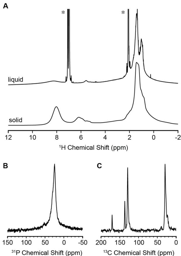
Fig. 3 NMR spectra of 19.8 nm ODPA-capped MOFs. (A) Liquid phase (top) and solid state (bottom)  $^1\text{H}$  NMR spectra. Asterisk (\*) denotes residual protonated solvent signals. (B)  $^{31}\text{P}$  solution phase NMR spectrum (50 Hz apodization applied). (C)  $^{13}\text{C}$  solid-state NMR spectrum.
