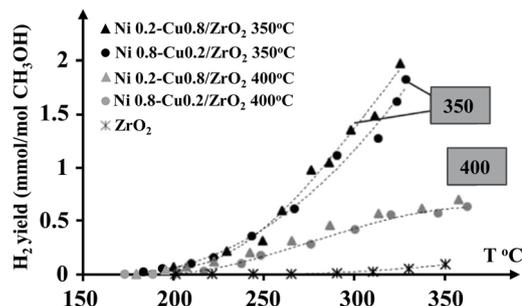
Fig. 1 H<sub>2</sub> yields of different ratios of Ni-Cu catalysts.<sup>23</sup> Reproduced from ref. 23 with permission from Elsevier, Copyright 2015.
