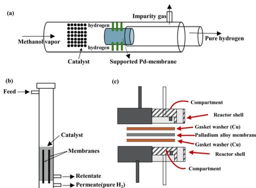
Fig. 6 Schematic representations of MRs with the (a) ceramic supported Pd membrane,<sup>84</sup> (b) Pd–Ag metallic active layer,<sup>87</sup> and (c) Pd–Cu alloy membrane.<sup>101</sup> (a) Reproduced from ref. 84 with permission from Elsevier, Copyright 2023. (b) Reproduced from ref. 87 with permission from Elsevier, Copyright 2022. (c) Reproduced from ref. 101 with permission from Pleiades Publishing Ltd, Copyright 2020.
