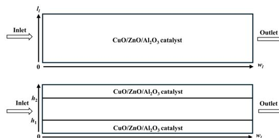
Fig. 5 Schematic representation of the reforming reactor: (a) packed bed and (b) coated-wall packed bed microreactors.<sup>78</sup> Reproduced from ref. 78 with permission from the Royal Society of Chemistry.
