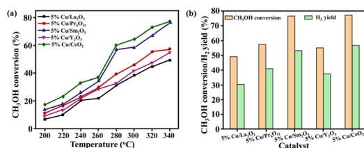
Fig. 2 Catalytic MSR reaction tests. (a) MeOH conversion and (b) H<sub>2</sub> yield at 340 °C.<sup>30</sup> Reproduced from ref. 30 with permission from Elsevier, Copyright 2023 Elsevier Ltd. All rights reserved.
