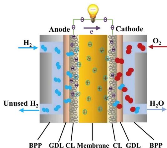
Fig. 7 PEMFC schematic illustration.<sup>121</sup> Reproduced from ref. 121 with permission from Elsevier, Copyright 2023.
