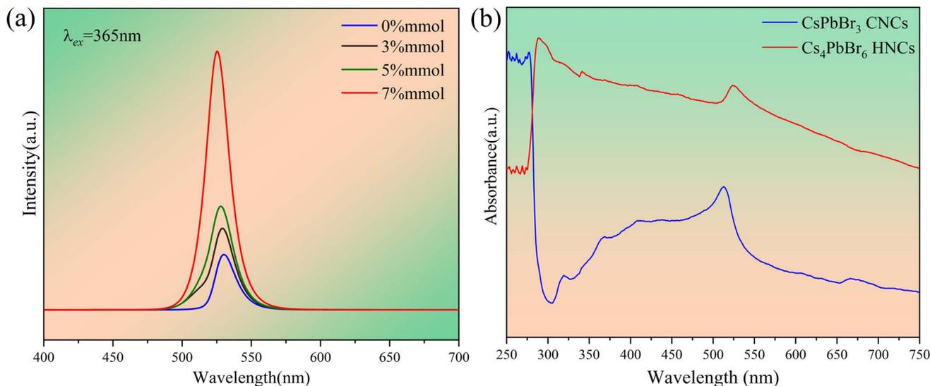
Fig. 4 (a) Emission spectra of CsPbBr<sub>3</sub> CNCs and Cs<sub>4</sub>PbBr<sub>6</sub> HNCs doped with PbS with different molar ratios. (b) Absorption spectra of CsPbBr<sub>3</sub> CNCs and Cs<sub>4</sub>PbBr<sub>6</sub> HNCs.
