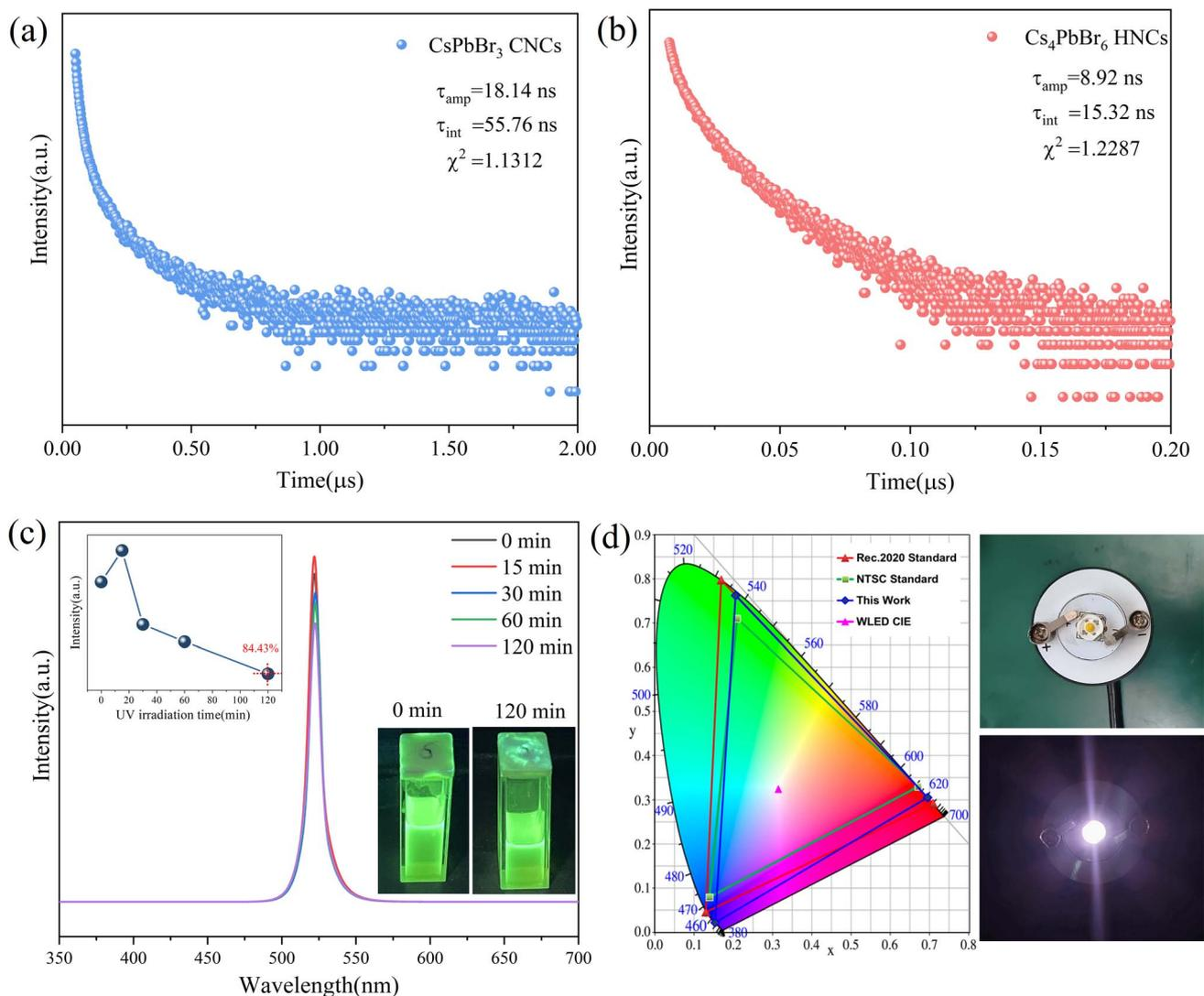
Fig. 5 (a) CsPbBr<sub>3</sub> CNCs fluorescence lifetime decay curve. (b) Cs<sub>4</sub>PbBr<sub>6</sub> HNCs fluorescence lifetime decay curve. (c) UV spectral stability of Cs<sub>4</sub>PbBr<sub>6</sub> HNCs under different time UV irradiation. (d) Cs<sub>4</sub>PbBr<sub>6</sub> HNCs backlight white LED package diagram and CIE diagram.
