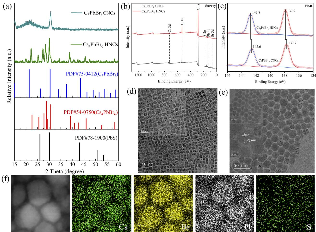
Fig. 2 (a) X-ray diffraction (XRD) patterns of Cs<sub>4</sub>PbBr<sub>6</sub> HNCs and CsPbBr<sub>3</sub> CNCs. (b) The full spectra of Cs<sub>4</sub>PbBr<sub>6</sub> HNCs and CsPbBr<sub>3</sub> CNCs. (c) Pb4f absorption peak spectra of Cs<sub>4</sub>PbBr<sub>6</sub> HNCs and CsPbBr<sub>3</sub> CNCs. (d and e) Are TEM spectra of Cs<sub>4</sub>PbBr<sub>6</sub> HNCs and CsPbBr<sub>3</sub> CNCs, respectively. (f) Analysis of TEM-EDS distribution of Cs<sub>4</sub>PbBr<sub>6</sub>.
