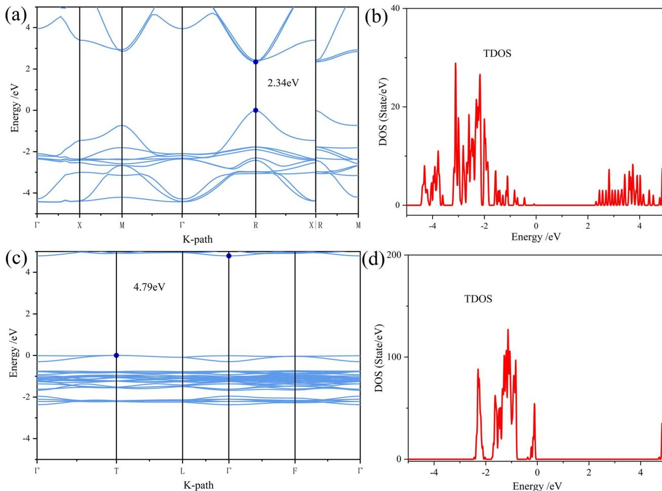
Fig. 3 The electronic band structures (a) and TDOS (b) of CsPbBr<sub>3</sub>; the electronic band structures (c) and TDOS (d) of Cs<sub>4</sub>PbBr<sub>6</sub> by density functional theory (DFT) calculations.
