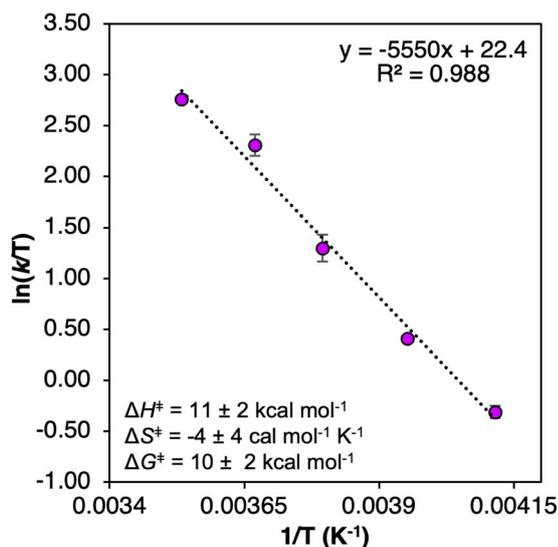
Fig. 4 Eyring plot of the PT from  $TiV_5O_6^{1-}$  and  $H_2Phen^{++}$  243–283 K in MeCN. Inset shows activation parameters. Error bars for each data point are determined from the standard deviation between three trials.
