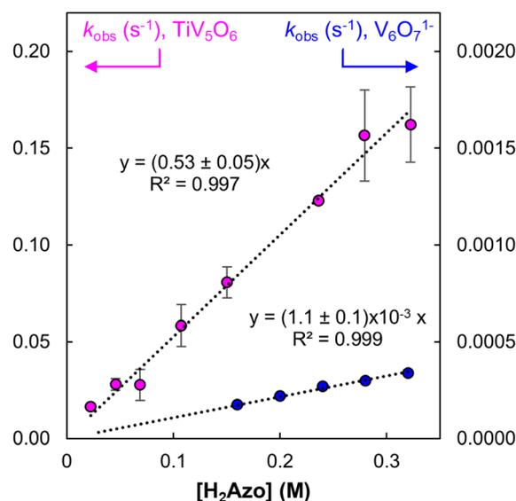
Fig. 7 Plot of  $k_{obs}$  as a function of  $[H_2Azo]$  for  $TiV_5O_6$  (pink circles, left Y-axis) and  $V_6O_7^{1-}$  (blue circles, right Y-axis) at 318 K. Concentration of POV were held constant at 0.75 mM, and reductant concentration was varied. The slope of the resultant lines provides the experimentally derived second-order rate constants,  $k_{exp}$ . Error bars for each data point are determined from the standard error of triplicate trials.
