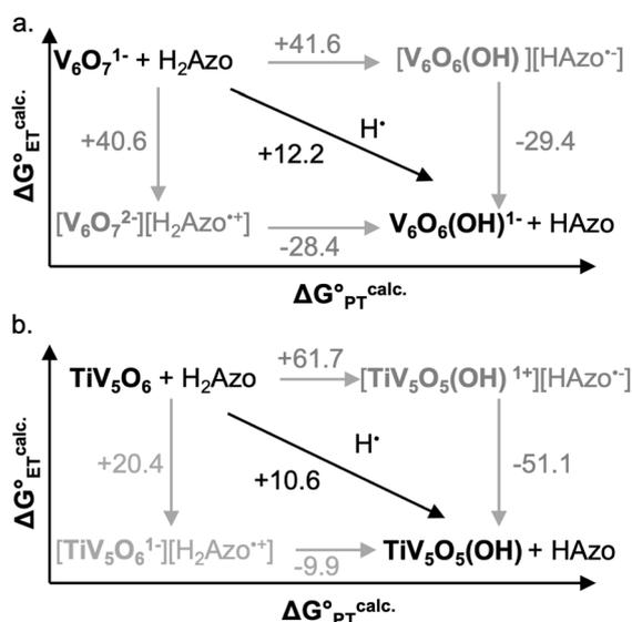
Fig. 9 Computationally derived thermochemistry of  $V_6O_7^{1-}$  (top, a) and  $TiV_5O_6$  species (bottom, b) with  $H_2Azo$ . Horizontal arrows are associated with PT free energies, vertical arrows with ET free energies, and diagonal arrows with CPET free energies. The black arrows represent the most favourable path from  $V^{V}=O$  to  $V^{IV}-OH$ . All presented energies are Gibbs free energies in kcal mol $^{-1}$ .
