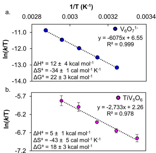
Fig. 8 Eyring plot of PCET from  $H_2Azo$  to  $V_6O_7^{1-}$  298–338 K in MeCN (top, a). Eyring plot of PCET from  $H_2Azo$  to  $TiV_5O_6$  308–348 K in MeCN (bottom, b). Inset shows activation parameters. Error bars for each data point are determined from the standard deviation between triplicate trials.
