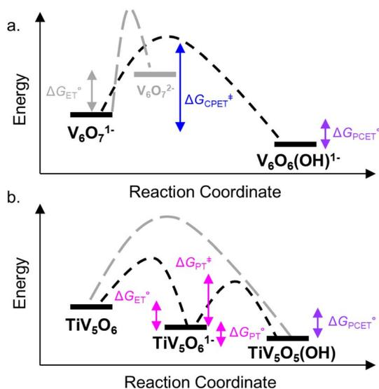
Fig. 3 Reaction coordinate diagram for reactivity of  $V_6O_7^{1-}$  (top, a) and  $TiV_5O_6$  (bottom, b) with  $H_2Phen$ . Activation energy for the CPET process is shown in blue traces. ET-PT free energy changes and PT activation energy are shown in pink traces. Free energy for PCET process is shown in purple. Grey traces show pathways that are not favourable. All values are listed in Table 1.
