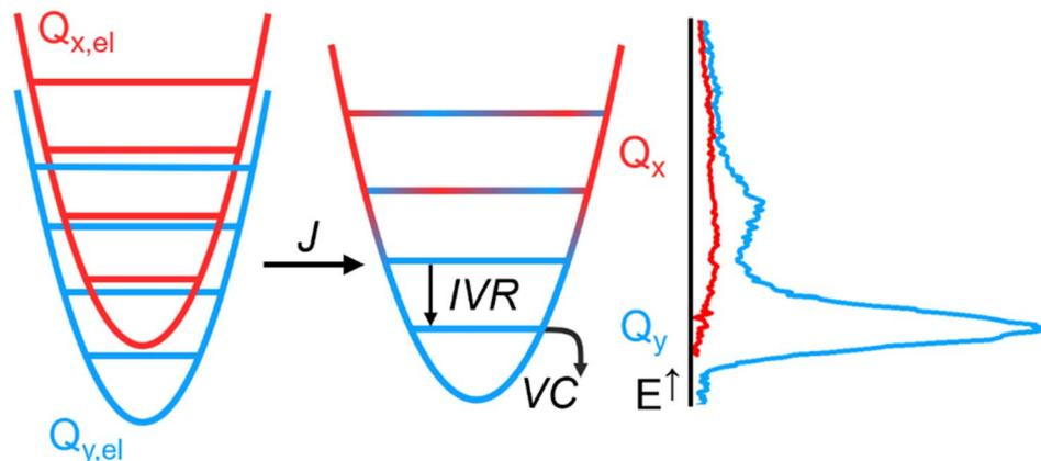
Fig. 5 Vibronic mixing ( $J$ ) in the Q band leads to strongly coupled states  $Q_x$  (red) and  $Q_y$  (blue). Ultrafast transfer *via*  $Q_x$  populates a vibrationally excited  $Q_y$ , which in turn relaxes *via* intra-molecular vibrational redistribution (IVR), followed by slower equilibration with the surrounding solvent (vibrational cooling VC). The right panel shows a sketch of the spectral profiles of  $Q_x$  and  $Q_y$ , as discussed in Fig. 1.
