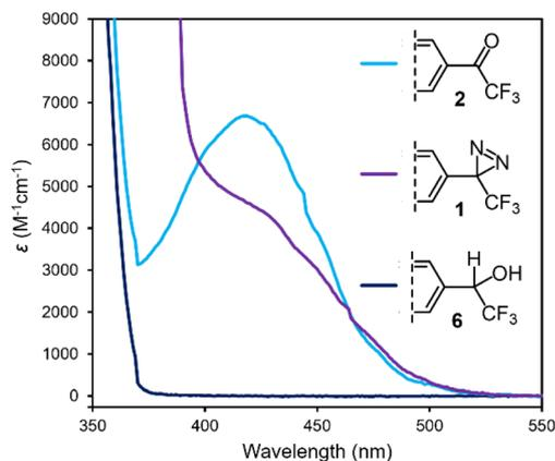
Fig. 8 UV/Vis spectrum for diazirine **1**, together with positive and negative control compounds **2** and **6**. All data were acquired using 0.05 mM samples in MeOH. Refer to the ESI† for UV/Vis data for compounds **1'**, **5**, and **7**, and for UV/Vis spectra collected in cyclohexane.
