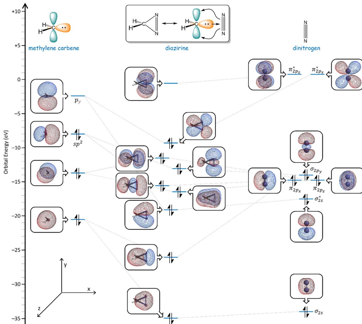
Fig. 11 Calculated frontier molecular orbitals (M06-2X/6-311+G(2df,2p)) for the parent diazirine molecule ( $\text{H}_2\text{CN}_2$ ), and correlations to the calculated orbitals of methylene carbene and dinitrogen.
