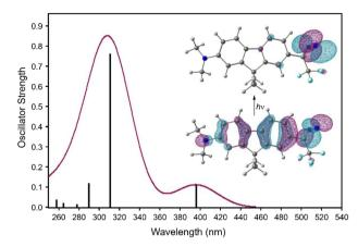
Fig. 9 TD-DFT calculated UV/Vis spectrum for diazirine 1. Geometry optimization and frequency calculations: M06-2X/6-31+G(d,p); TD-DFT: CAM-B3LYP/aug-cc-pVTZ with implicit methanol solvation. Inset figure shows natural transition orbitals<sup>30</sup> involved in the low-energy excitation.
