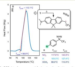
Fig. 6 DSC data for compound 1, showing the diazirine activation exotherm.  $T_{\rm peak}$  corresponds to the temperature at which the maximum heat flow is observed.  $T_{\rm onset}$  is determined experimentally from extrapolation of the tangent of the upward slope observed in the DSC experiment (red dotted line), to the fitted baseline of the plot. Inset data taken from ref. 17 show the decrease in activation temperature with increasing electron density in the aromatic ring.
