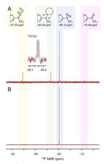
Fig. 10  $^{19}$ F NMR spectra illustrating the activation of diazirine 1 using near-IR light. (A) NMR spectrum following irradiation of 1 in cyclohexane with 815 nm light. (B) Control sample stored in an amber vial. The inset shows a  $^{1}$ H-coupled  $^{19}$ F NMR spectrum, which confirms the presence of cyclohexane adduct 7.
