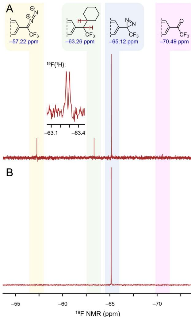
Fig. 10  $^{19}\text{F}$  NMR spectra illustrating the activation of diazirine **1** using near-IR light. (A) NMR spectrum following irradiation of **1** in cyclohexane with 815 nm light. (B) Control sample stored in an amber vial. The inset shows a  $^1\text{H}$ -coupled  $^{19}\text{F}$  NMR spectrum, which confirms the presence of cyclohexane adduct **7**.
