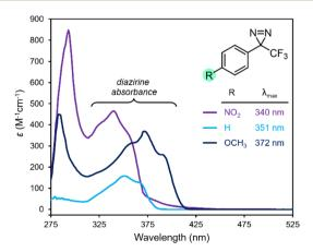
Fig. 2 Changes in UV/Vis absorption spectra with varying substitution on the aromatic ring of a trifluoromethyl aryl diazirine. All data were acquired using 5 mM samples in n-hexane. Replotted from raw data published in ref. 17.
