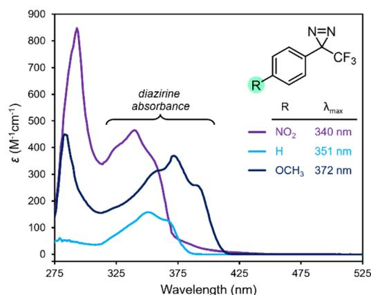
Fig. 2 Changes in UV/Vis absorption spectra with varying substitution on the aromatic ring of a trifluoromethyl aryl diazirine. All data were acquired using 5 mM samples in *n*-hexane. Replotted from raw data published in ref. 17.
