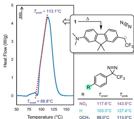
Fig. 6 DSC data for compound 1, showing the diazirine activation exotherm.  $T_{\text{peak}}$  corresponds to the temperature at which the maximum heat flow is observed.  $T_{\text{onset}}$  is determined experimentally from extrapolation of the tangent of the upward slope observed in the DSC experiment (red dotted line), to the fitted baseline of the plot. Inset data taken from ref. 17 show the decrease in activation temperature with increasing electron density in the aromatic ring.
