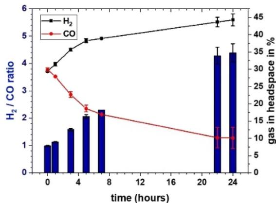
Fig. 7 Evolution of the proportions of  $\text{H}_2$  and CO detected by GC in the headspace of a WGSR experiment over time and its corresponding  $\text{H}_2/\text{CO}$  ratio (vial flushed with syngas mix (30% CO, 30%  $\text{H}_2$ , 20%  $\text{CO}_2$ , 10%  $\text{CH}_4$ , 10%  $\text{N}_2$  at  $t_0$ , corresponding to 7 mL gas mix at ambient pressure and  $25^\circ \text{C}$ ,  $0.9 \text{ nmol per cm}^2$  Rec-RrCODH and  $110 \text{ nmol per cm}^2$  NiPNP<sup>Arg</sup>)).
