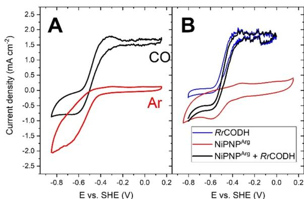
Fig. 3 (A) CV of the bifunctionalized MWCNT electrode under Ar and CO in 50 mM Bis-Tris propane buffer pH 7.0 ( $v = 5$  mV s<sup>-1</sup>); (B) CV of the **Rec-RrCODH**-modified MWCNT electrode (blue) and **NiPNP<sup>Arg</sup>**-modified MWCNT electrode (red) under CO in 50 mM Bis-Tris propane buffer pH 7.0 ( $v = 5$  mV s<sup>-1</sup>) and the corresponding sum of both CV (black, capacitive contribution of one CV was removed).
