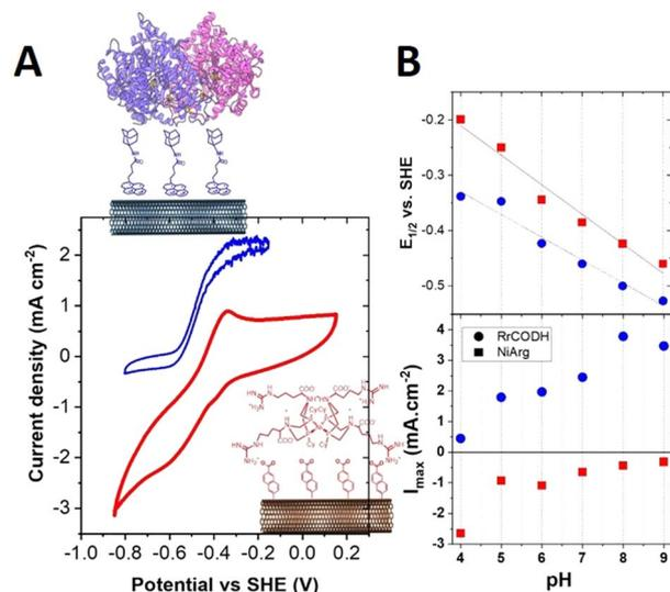
Fig. 2 (A) Cyclic voltammetry (CV) of NiPNP<sup>Arg</sup>-modified N<sup>A</sup>MWCNT electrode (red) under Ar, and Rec-RrCODH modified ADAMWCNT electrode (blue) under CO in 50 mM Bis-Tris propane buffer pH 7.0 ( $v = 5 \text{ mV s}^{-1}$ ): (B) half-wave potential and  $I_{\text{max}}$  versus pH for NiPNP<sup>Arg</sup>-modified MWCNT electrode (red) under Ar, and Rec-RrCODH-modified MWCNT electrode (blue) under CO in 50 mM Bis-Tris propane buffer pH 7.0.
