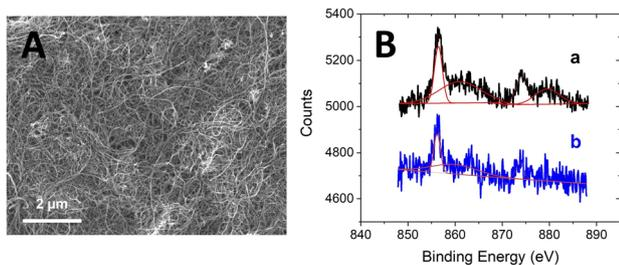
Fig. 6 (A) SEM micrograph and (B) XPS spectra of Ni 2p core energy levels for MWCNT film modified with both NiPNP<sup>Arg</sup>- and Rec-RrCODH before (a) and after (b) 24 h WGSR accompanied with XPS simulation (red line).
