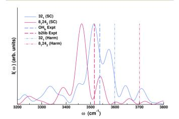
Fig. 2 Semiclassical calculations of the hydrogen-bonded water OH<sub>b</sub> stretch (32<sub>1</sub>, blue) and b2lib combination band (8<sub>1</sub>24<sub>2</sub>, pink) for acetone monohydrate. The zero of energy is set at the ZPE, so that I(E)is replaced by  $I(\omega)$ .
