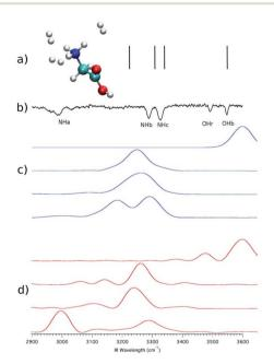
Fig. 1 Vibrational spectra for protonated glycine microsolvated by three H<sub>2</sub> molecules. Panel (a): harmonic estimates. Panel (b): the experimental spectrum; Panel (c): the quasi-classical trajectory method results; Panel (d): DC-SCIVR calculation. This figure has been reproduced from ref. 47 with permission from the Royal Society of Chemistry, copyright 2018.
