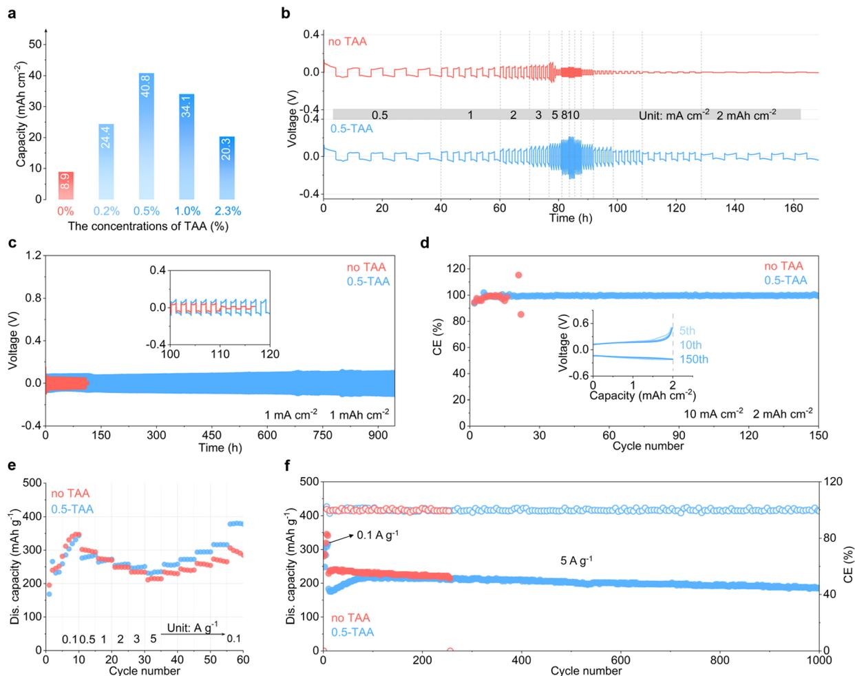
Fig. 4 Electrochemical performance of the Zn electrode in the 2 m ZnSO<sub>4</sub> electrolyte without and with 0.5 wt% TAA additive: (a) single deposition capacity with different TAA percentages; (b) rate performance and (c) long-term cycling stability of symmetric Zn cells; (d) coulombic efficiencies of Zn//Cu cells; (e) rate performance and (f) long-term cycling performance of Zn//V<sub>2</sub>O<sub>5</sub> cells.
