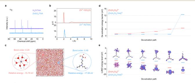
Fig. 2 (a)  $^{13}$ C NMR of 0.5 wt% TAA without and with ZnSO<sub>4</sub> salt. (b) RDFs, (c) MD simulation box, together with the structures, relative energies and bond orders of  $[Zn(H_2O)_6]^{2+}$  and  $[Zn(H_2O)_5TAA]^{2+}$  solvation structures in the ZnSO<sub>4</sub> electrolyte with 0.5 wt% TAA additive. (d) Desolvation energy barriers at each step and (e) corresponding LUMO energy levels of  $[Zn(H_2O)_6]^{2+}$  and  $[Zn(H_2O)_5TAA]^{2+}$ .
