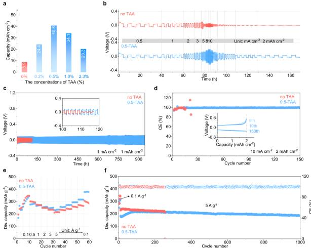
Fig. 4 Electrochemical performance of the Zn electrode in the 2 m ZnSO<sub>4</sub> electrolyte without and with 0.5 wt% TAA additive: (a) single deposition capacity with different TAA percentages; (b) rate performance and (c) long-term cycling stability of symmetric Zn cells; (d) coulombic efficiencies of Zn//Cu cells; (e) rate performance and (f) long-term cycling performance of Zn// $V_2O_5$  cells.
