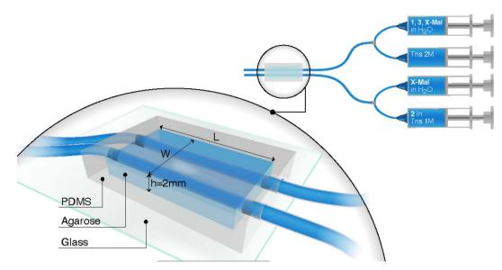
Fig. 2 Scheme of the experimental set-up. Reagents are supplied to the gel reactor from three or four syringes. The magnified image of the gel reactor is shown in three-dimensional projection. The images of the gel are recorded from the top by USB camera. X-Mal stands for Mal, TPEG-Mal, and HPEG-Mal.
