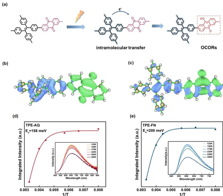
Fig. 4 Generation process of OCORs. (a) Schematic diagram of oxygen-centered organic radical (OCOR) generation. (b and c) The analysis of the distribution of holes (blue) and electrons (green) for TPE-AQ (b) and TPE-FN (c) using TD-DFT calculations. (d and e) Temperature-dependent PL spectra of (d) TPE-AQ and (e) TPE-FN; inset: evolution of PL intensity as a function of temperature for (d) TPE-AQ and (e) TPE-FN.
