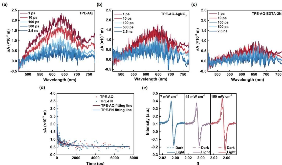
Fig. 5 Generation process and mechanism of OCORs. (a–c) The transient absorption spectra of TPE-AQ with different quenchers. TA values of CPs pumped at 400 nm for  $\text{AgNO}_3$  and EDTA-2Na were all 10 mM. (d) TA kinetic traces of TPE-AQ and TPE-FN in  $\text{H}_2\text{O}$  probed at 634 nm and 615 nm, respectively. (e) Spectrogram of EPR signal intensity as a function of excitation light intensity.
