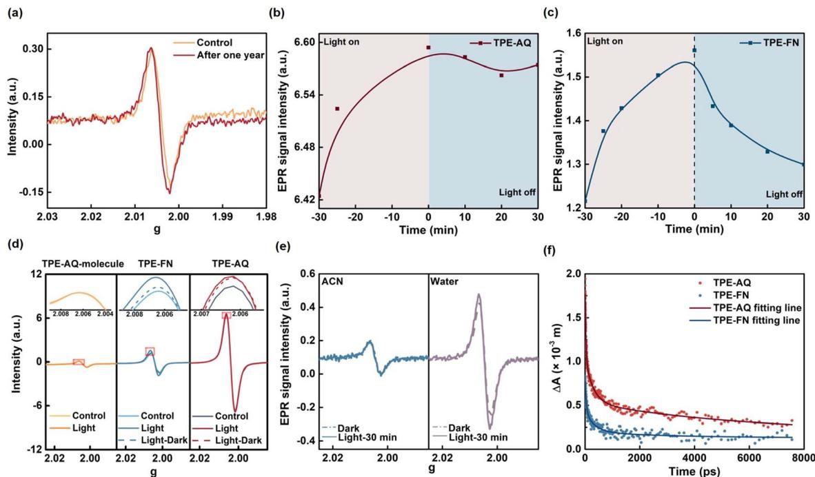
Fig. 6 Stability mechanism for OCORs. (a) EPR spectra before and after TPE-AQ placement for one year. (b–d) The time-dependent *in situ* solid EPR spectra of TPE-AQ (b) and TPE-FN (c), and (d) the EPR spectrum and (b and c) the highest point of EPR signal intensity as the ordinate ( $g = 2.0063$ ). (e) EPR spectra of TPE-AQ in water and acetonitrile before and after light irradiation. (f) TA kinetic traces of TPE-AQ and TPE-FN in  $H_2O$  probed at 1110 nm and 972 nm, respectively.
