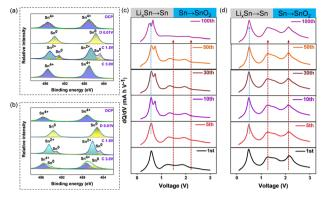
Fig. 2 Ex situ XPS spectra of Sn 3d for (a) NSM and (b)  $SnO_2$  at four different charge states. Differential charge capacity versus voltage plots for (c)  $SnO_2$  and (d) NSM electrodes from the 1st to the 100th cycles.
