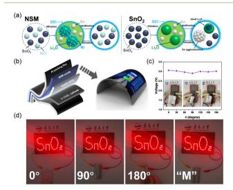
Fig. 5 (a) Schematic diagram of the electrochemical performance mechanism of NSM and SnO<sub>2</sub> electrodes. (b) Structure model of a thin film battery and photographs of an electrochromic watch powered by a flexible battery. (c) Open circuit voltage and (d) an LED logo of SnO<sub>2</sub> powered by a flexible quasi-solid-state pouch cell at varied folding levels
