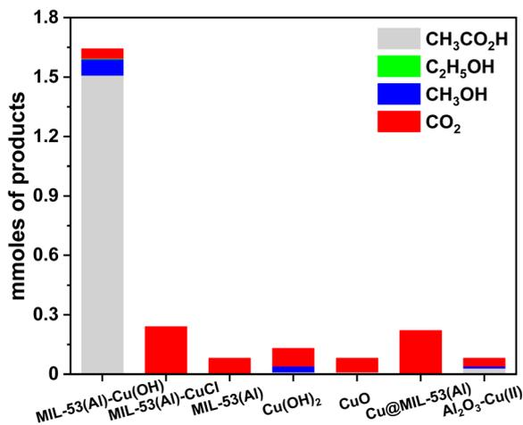
Fig. 5 Comparison of the catalytic efficiency of MIL-53(Al)-Cu(OH) with other materials in direct methane oxidation to acetic acid under identical reaction conditions. Conditions: 30 bar CH<sub>4</sub>, 10 bar O<sub>2</sub>, 175 °C and 32 h.
