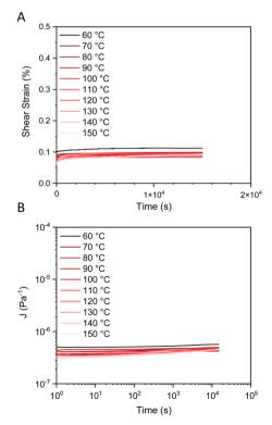
Fig. 7 Strain vs. time (A) and creep compliance with time (B) plots for the R0 materials containing 5%-NPC2.
