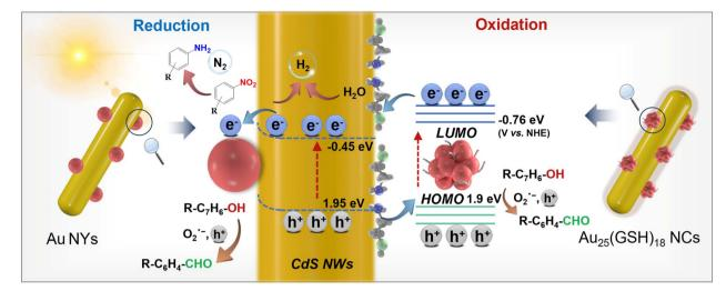
Scheme 1 Schematic illustration depicting the photoredox mechanisms of CdS/Au<sub>25</sub>(GSH)<sub>18</sub> and CdS/Au heterostructures.
