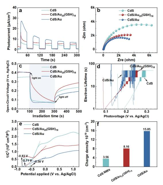
Fig. 5 PEC water splitting performances of CdS NWs, CdS/Au<sub>25</sub>(GSH)<sub>18</sub> and CdS/Au heterostructures in Na<sub>2</sub>SO<sub>4</sub> aqueous solution (pH = 6.69) under visible light irradiation ( $\lambda$  > 420 nm) including (a) transient photocurrent responses (bias: 0.61 V vs. RHE), and (b) EIS results, (c) OCVD & (d) electron lifetime, and (e) Mott–Schottky plots & (f) charge carrier density ( $N_D$ ).
