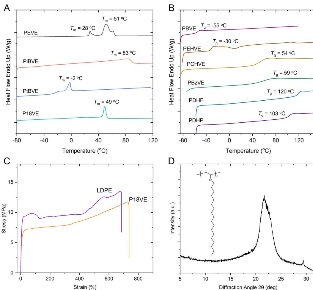
Fig. 4 (A) and (B) DSC results of poly(vinyl ether) polymers obtained. PEVE with 81% *m* was tested. Data are rescaled and shifted vertically for clarity. (C) Stress vs. strain curves for P18VE with 75% *m* and LDPE. (D) XRD pattern of the P18VE film.
