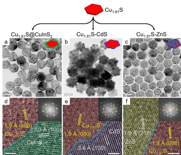
Fig. 2 CE reactions on  $\text{Cu}_{1.81}\text{S}$  nanoplates. TEM and HRTEM images of different CE reaction products obtained through (a and d)  $\text{In}^{3+}$ , (b and e)  $\text{Cd}^{2+}$ , and (c and f)  $\text{Zn}^{2+}$  exchange, respectively. For convenience, HRTEM images are colored according to different metal sulfide domains. The colors correspond to the circles in the FFT patterns of the insets. Scale bars: (a–c) 100 nm; (d–f) 2 nm.
