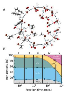
Fig. 2 (A) Proposed overall reaction pathway of CO<sub>2</sub> hydrogenation over iron-based catalysts. Adapted from ref. 44; and (B) iron-phase composition as a function of time during Fischer-Tropsch synthesis determined by Mössbauer spectroscopy over a Fe-Cu/K/Al catalyst. Adapted from ref. 45.
