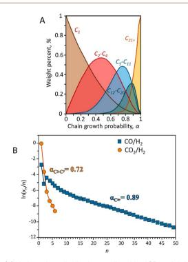
Fig. 3 (A) Hydrocarbon distribution predicted by ASF model. Adapted from ref. 53 and (B) hydrocarbons experimental ASF plots reported in terms of selectivity during CO and  $\rm CO_2$  hydrogenation. Adapted from ref. 54.
