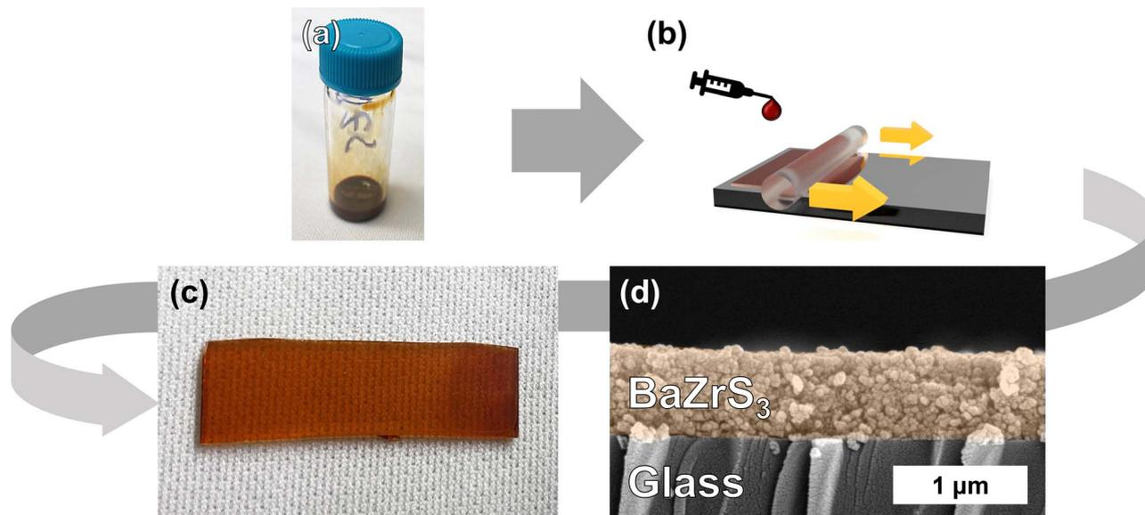
Fig. 5 Blade coating procedure to produce BaZrS<sub>3</sub> nanoparticle films. (a) Shows a typical ink of suspended BaZrS<sub>3</sub> nanoparticles, (b) illustrates the blade coating procedure, (c) shows a photograph of the coated film on a glass substrate, and (d) shows a cross-section SEM image of the same film.
