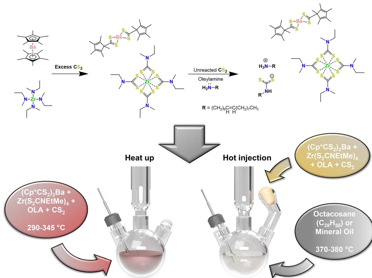
Scheme 1 Precursor preparation and experimental protocol for BaZrS<sub>3</sub> nanoparticle syntheses. Sr and Ti/Hf analogues were used in place of Ba and Zr, respectively, for BaTiS<sub>3</sub>, BaHfS<sub>3</sub>, SrZrS<sub>3</sub>, and SrHfS<sub>3</sub> nanocrystal syntheses. Reaction ware setup is also illustrated (bottom).
