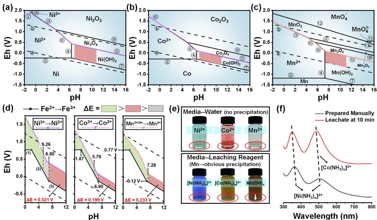
Fig. 1 The Pourbaix diagram of the (a) Ni–H<sub>2</sub>O system, (b) Co–H<sub>2</sub>O system, and (c) Mn–H<sub>2</sub>O system. (d) The partial area comparison of the Fe–H<sub>2</sub>O system with Ni, Co, and Mn–H<sub>2</sub>O systems. (e) The real picture of the three metal ions in different solutions. (f) The UV-vis spectra of the leachate and control group.
