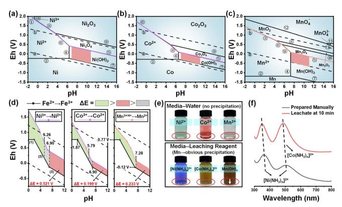
Fig. 1 The Pourbaix diagram of the (a) Ni-H<sub>2</sub>O system, (b) Co-H<sub>2</sub>O system, and (c) Mn-H<sub>2</sub>O system. (d) The partial area comparison of the Fe-H<sub>2</sub>O system with Ni, Co, and Mn-H<sub>2</sub>O systems. (e) The real picture of the three metal ions in different solutions. (f) The UV-vis spectra of the leachate and control group
