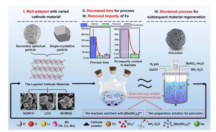
Fig. 7 The advantages of alkaline leaching in the recycling of spent cathode materials
