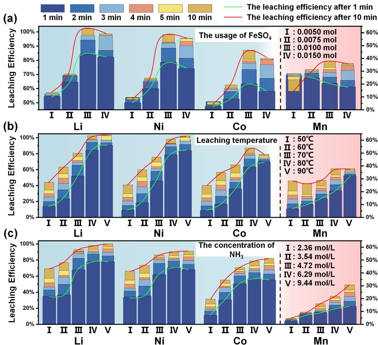
Fig. 3 The leaching efficiency of valuable metals changes with the gradient of (a) FeSO<sub>4</sub> usage, (b) leaching temperature, and (c) the concentration of NH<sub>3</sub>.
