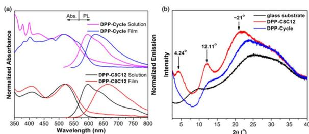
Fig. 5 (a) UV-vis absorption and fluorescence spectra of **DPP-C8C12** and **DPP-Cycle** in dilute trichlorobenzene solution and in thin films. (b) XRD patterns of **DPP-C8C12** and **DPP-Cycle** thin films measured on a glass substrate.
