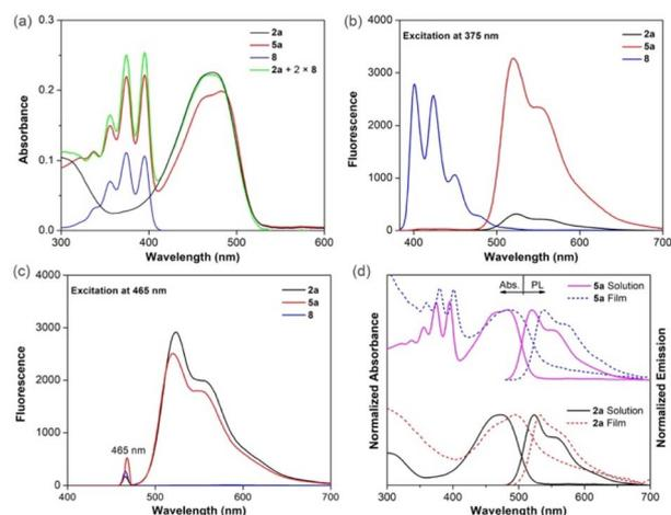
**Fig. 3** (a) UV-vis absorption spectra of **2a**, **5a** and **8** in chloroform (10  $\mu$ M). Fluorescence spectra of **2a**, **5a** and **8** in chloroform (1  $\mu$ M) recorded upon excitation of the anthracene chromophore at 375 nm (b) and excitation of the DPP chromophore at 465 nm (c). (d) Normalized UV-vis absorption spectra and emission spectra of **2a** and **5a** in chloroform solution (solid line) and as thin films (dashed line).
