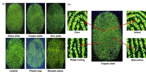
Fig. 7 (a) Fluorescent images of LFPs developed using **5a**@silica on different substrate surfaces. (b) Secondary level information visible when a copper plate was used as the substrate with the LFP subjected to digital magnification.
