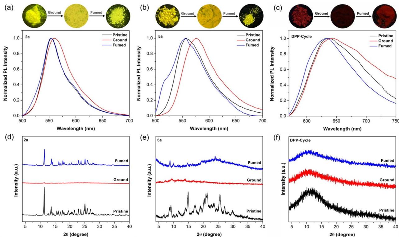
Fig. 6 The fluorescence spectra of solid powders of **2a** (a), **5a** (b) and **DPP-Cycle** (c) studied in different solid state forms. Top: Corresponding fluorescence images recorded under a 365 nm ultraviolet lamp. The corresponding PXRD patterns of **2a** (d), **5a** (e) and **DPP-Cycle** (f) recorded in different solid state forms.
