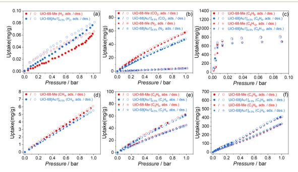
Fig. 2 Single-component sorption isotherms for (a)  $H_2$ , (b)  $CO_2$  and  $N_2$ , (c)  $C_6H_6$  and  $C_6H_{12}$ , (d)  $CH_4$ , (e)  $C_2H_4$  and  $C_2H_6$ , and (f)  $C_3H_6$  and  $C_3H_8$  of UiO-68-Me and UiO-68[Au1]<sub>4.5%</sub> at 298.15 K. "Ads" and "des" stand for adsorption and desorption, respectively.
