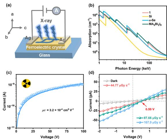
Fig. 3 (a) The device fabrication of the Ag |1 SC| Ag with the electrode direction parallel to the *c*-axis; (b) calculated absorption spectra of 1, Si,  $\alpha$ -Se, and  $\text{MA}_3\text{Bi}_2\text{I}_9$ ; (c) Bias-dependent photoconductivity of 1; (d)  $I$ - $V$  curves of the 1 device along the *c*-axis in the dark and under X-ray irradiation.
