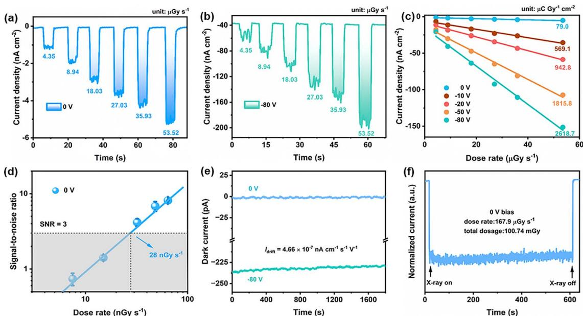
Fig. 4 (a and b) Photoresponses of the 1 detector to X-rays at increased dose rates at 0 and  $-80 \text{ V}$  bias, respectively; (c) X-ray photocurrent density as a function of the dose rate; (d) X-ray dose rate dependent SNR at zero bias; (e) the dark current drift at  $-80 \text{ V}$  bias; (f) the stable photoresponse of the 1 device resisting X-ray irradiation.
