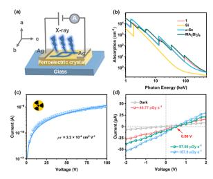
Fig. 3 (a) The device fabrication of the Ag  $|1\ SC|$  Ag with the electrode direction parallel to the c-axis; (b) calculated absorption spectra of 1, Si,  $\alpha$ -Se, and MA $_3$ Bi $_2$ I $_9$ ; (c) Bias-dependent photoconductivity of 1; (d) I-V curves of the 1 device along the c-axis in the dark and under X-ray irradiation
