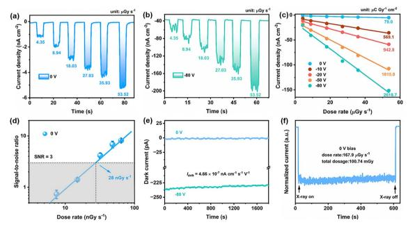
Fig. 4 (a and b) Photoresponses of the 1 detector to X-rays at increased dose rates at 0 and -80 V bias, respectively; (c) X-ray photocurrent density as a function of the dose rate; (d) X-ray dose rate dependent SNR at zero bias; (e) the dark current drift at -80 V bias; (f) the stable photoresponse of the 1 device resisting X-ray irradiation.
