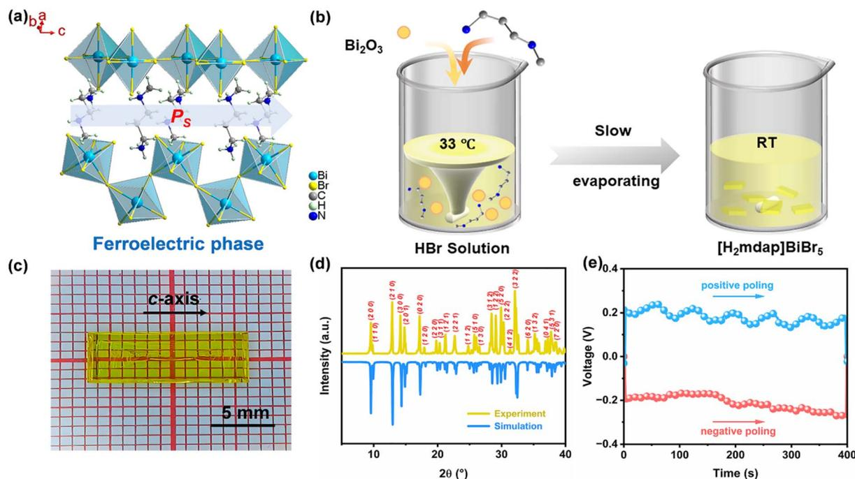
Fig. 1 (a) The crystal structure of **1** in the ferroelectric phase; (b) schematic for the growth of the **1** crystal; (c) a photograph for the **1** SC; (d) the experimental and simulated powder XRD patterns; (e) *V*–*t* curves along the *c*-axis, measured after positive and negative polings.
