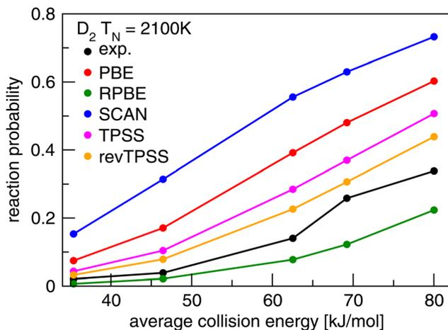
Fig. 6 Values of  $S_0$  measured<sup>78</sup> in molecular beam experiments for  $D_2 + Cu(111)$  are compared to computed<sup>79</sup> values using PESs based on DFT calculations using the GGA PBE<sup>80</sup> and RPBE<sup>48</sup> DFs, and the *meta*-GGA SCAN,<sup>81</sup> TPSS,<sup>82</sup> and rev-TPSS<sup>83</sup> DFs. Figure taken from ref. 79 (<https://doi.org/10.1021/acs.jpca.9b02914>). Further permission requests to be directed to the ACS.
