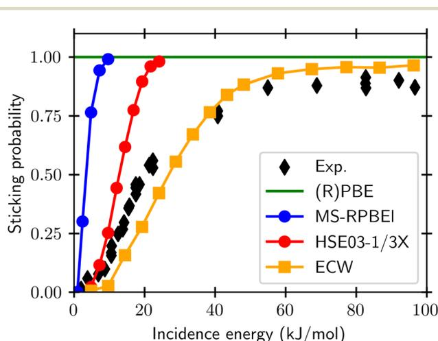
Fig. 9 Sticking probabilities computed with the GGA PBE and RPBE DFs,<sup>51,52</sup> the *meta*-GGA MS-RPBEI DF,<sup>41</sup> the screened hybrid HSE03-1/3X DF,<sup>41</sup> and with embedded correlated wave function theory<sup>95</sup> are compared with experimental results, for sticking of  $O_2$  on  $Al(111)$ .<sup>96</sup> Figure taken from ref. 41 (<https://pubs.acs.org/doi/10.1021/acs.jpcllett.0c02452>). Further permission requests to be directed to the ACS.
