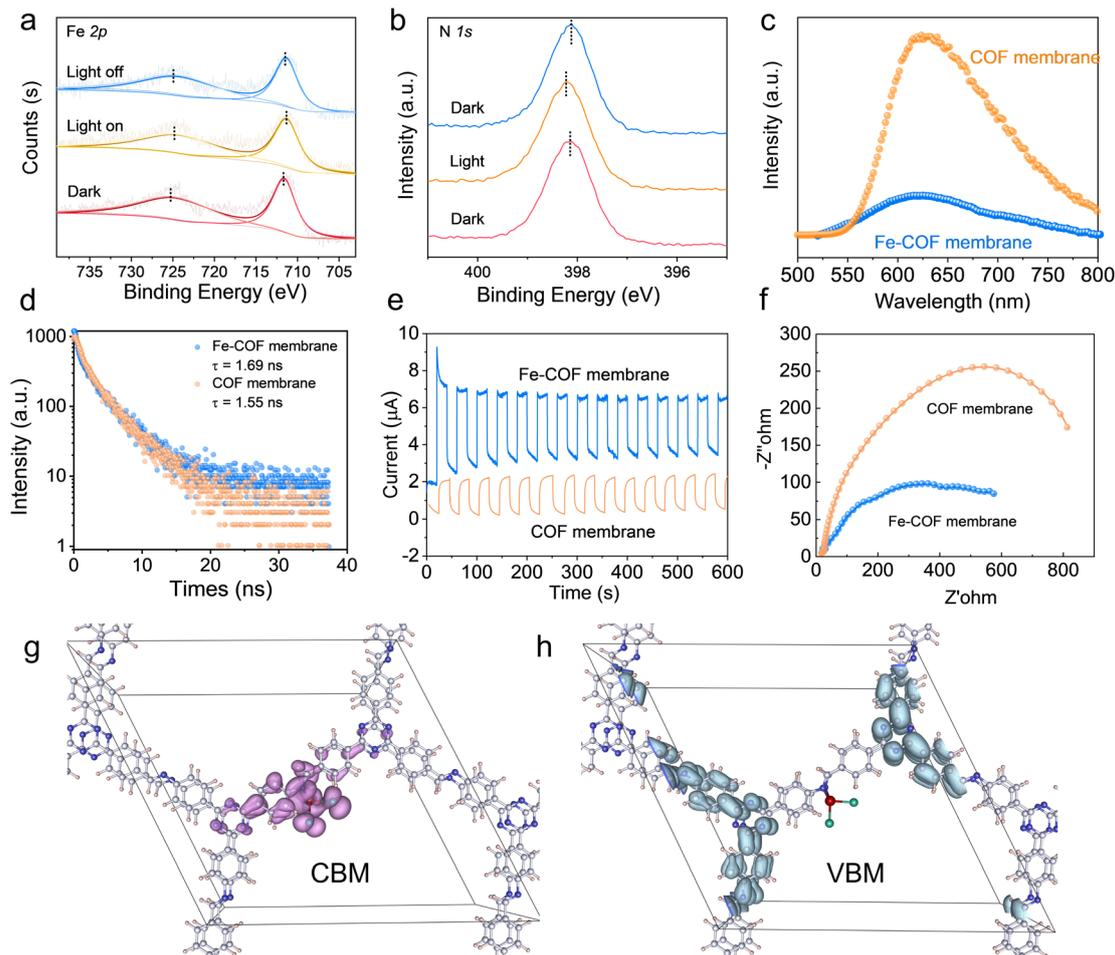
Fig. 6 (a and b) *In situ* high-resolution XPS spectra. (c) Photoluminescence intensity. (d) Photoluminescence lifetime. (e) Photocurrent density. (f) Charge transfer resistance of different COF membranes. (g) The CBM and (h) VBM of the Fe-COF membrane.
