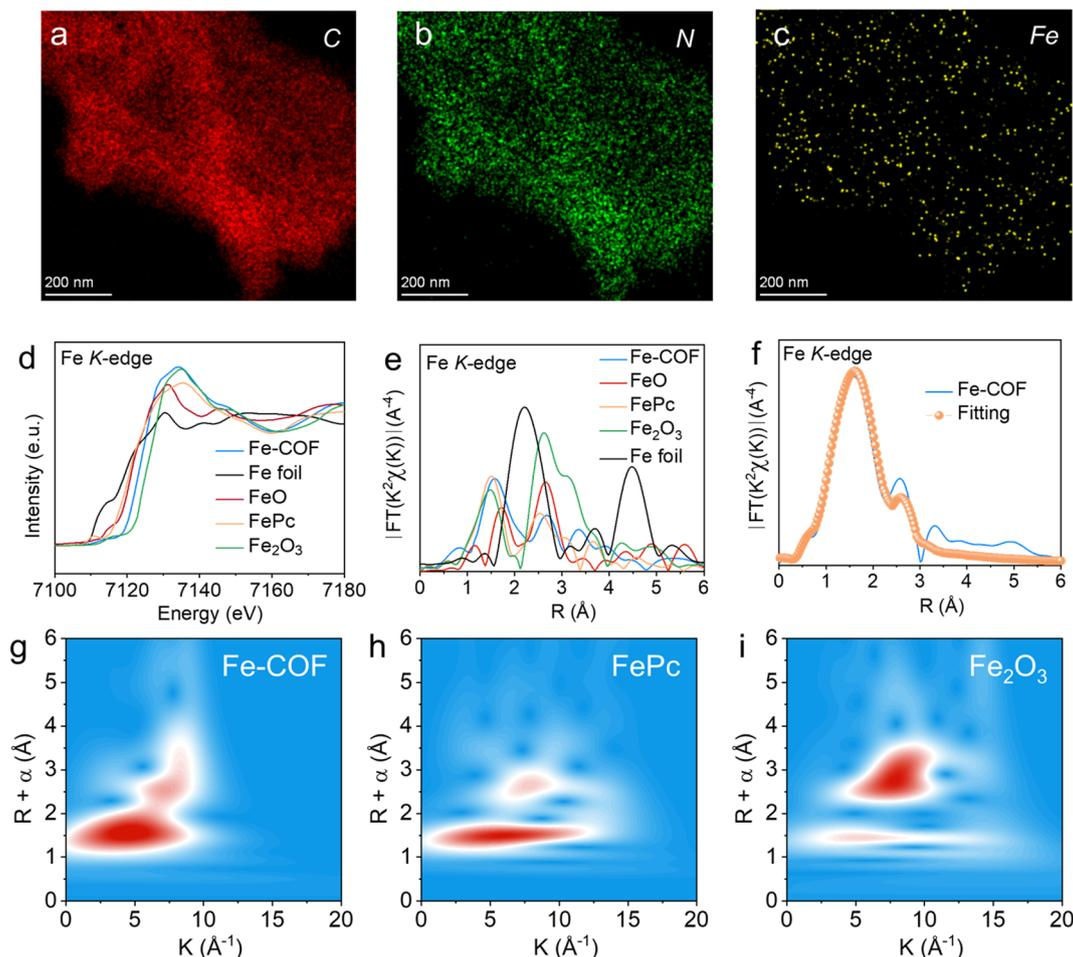
Fig. 3 (a–c) Element mapping of the Fe–COF membrane. (d) Normalized XANES and (e) Fourier-transformed (FT) EXAFS spectra at the Fe K-edge. (f) The EXAFS fitting curves of the Fe–COF membrane in  $R$  space. The WT-EXAFS spectra of (g) the Fe–COF membrane, (h) FePc, and (i)  $\text{Fe}_2\text{O}_3$ .
