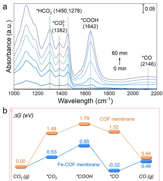
Fig. 7 (a) *In situ* DRIFTS of the Fe-COF membrane during the CO<sub>2</sub> photoreduction process. (b) Free energy profile of the CO<sub>2</sub>RR to CO catalyzed by the Fe-COF and the pristine COF membranes.
