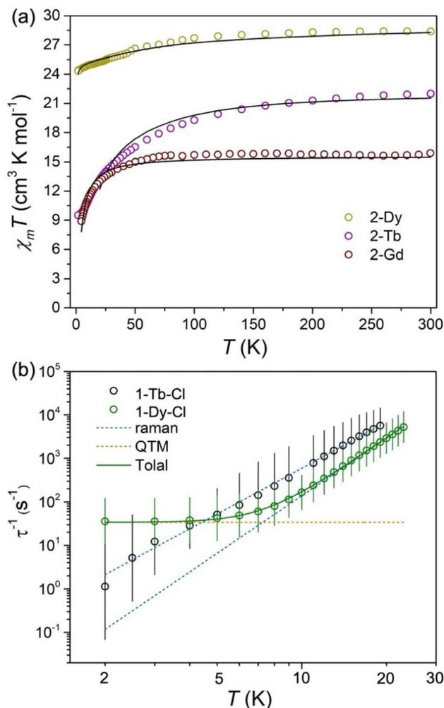
Fig. 6 (a) Temperature dependent susceptibility of  $\chi_M T$  in an applied dc magnetic field of 1 kOe for 2-Dy, 2-Tb and 2-Gd. The black solid lines represent the best fit from *ab initio* calculations (2-Dy and 2-Tb) or eqn (1) (2-Gd). (b) Plot of natural log of the inverse relaxation time vs. temperature for 1-Tb-Cl and 1-Dy-Cl. The plots are from the ac susceptibility measurements with applied field (0 Oe for 1-Dy-Cl and 2 kOe for 2-Tb-Cl). The lines are the best fit.
