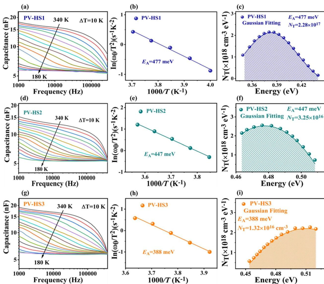
Fig. 6 Characterization of temperature-dependent admittance spectroscopy for Sb<sub>2</sub>(S,Se)<sub>3</sub> photovoltaic devices. (a, d and g) Variation of capacitance at different frequencies and temperatures. (b, e and h) Using the Arrhenius plots of the characteristic frequencies to acquire the defect activation energy. (c, f and i) Defect distributions of PV-HS1, PV-HS2 and PV-HS3 devices.
