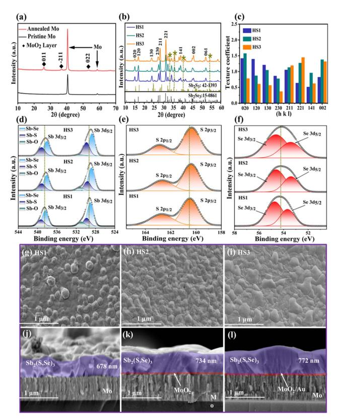
Fig. 2 (a) XRD patterns of pristine and post-annealed (400 °C/15 min) Mo substrates. (b) XRD patterns, (c) texture coefficients, and (d-f) XPS peaks of thin films from HS1, HS2 and HS3 samples. (g-i) SEM images of the surface morphology, and (j-l) cross-sectional SEM images of thin films from HS1, HS2 and HS3 samples.
