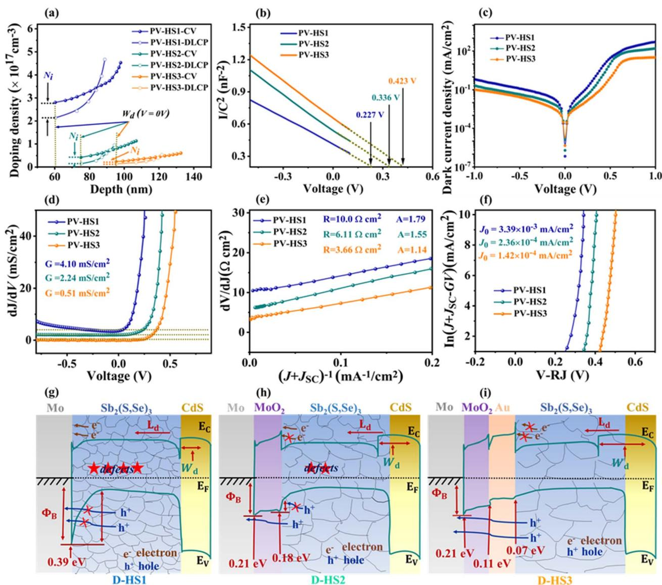
Fig. 7 (a) C-V and DLCP profiles. (b)  $1/C^2$ -V graphs of the PV-HS1, PV-HS2, and PV-HS3 photovoltaic devices. Electrical behaviours of the corresponding three devices: (c) dark  $J$ -V curves, (d) characterization of the shunt conductance  $G$ , (e) the series resistance  $R$ , the ideality factor  $A$ , and (f) the current density  $J_{\text{sc}}$  for reverse saturation. The band diagrams of D-HS1 (g), D-HS2 (h), and D-HS3 (i) devices.
