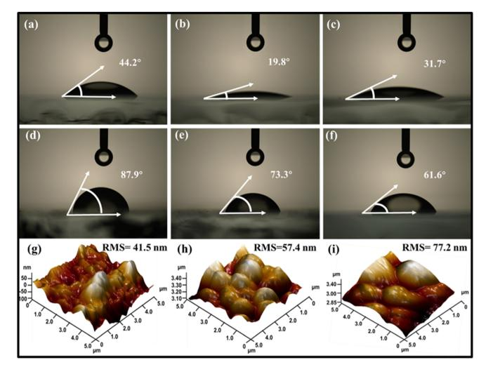
Fig. 1 (a-c) The measured CAs (using water droplets) of pristine Mo, post-annealed Mo at 400 °C/15 min, and post-annealed Mo sputtered with Au, respectively. (d-f) The measured CAs of the thin films from HS1, HS2, and HS3 samples and (q-i) the corresponding AFM topographical images of the thin films from HS1, HS2 and HS3 samples.
