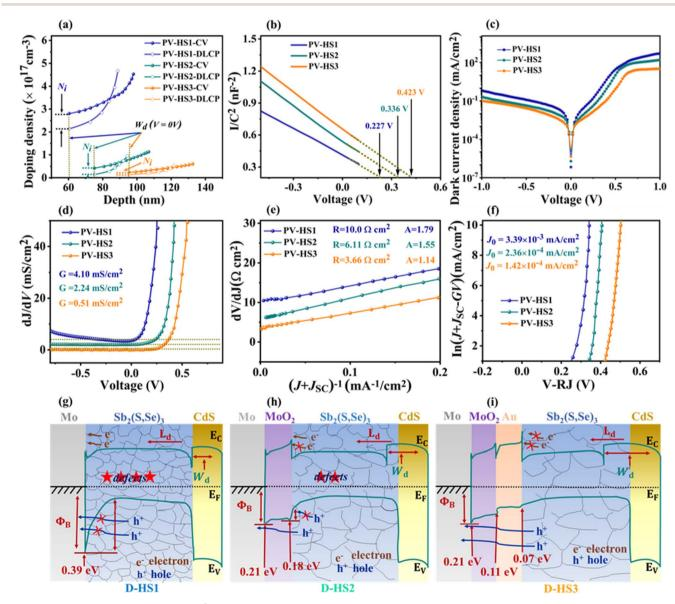
Fig. 7 (a) C-V and DLCP profiles. (b)  $1/C^2-V$  graphs of the PV-HS1, PV-HS2, and PV-HS3 photovoltaic devices. Electrical behaviours of the corresponding three devices: (c) dark J-V curves, (d) characterization of the shunt conductance G, (e) the series resistance R, the ideality factor A, and (f) the current density  $J_{sc}$  for reverse saturation. The band diagrams of D-HS1 (g), D-HS2 (h), and D-HS3 (i) devices.
