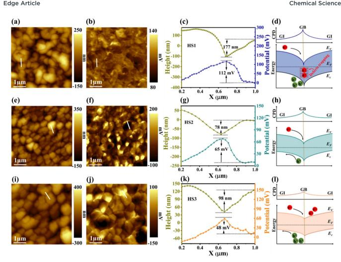
Fig. 3 KPFM characterization of thin films from HS1 (a-d), HS2 (e-h), and HS3 (i-l) samples. (a) Topography, (b) surface potential, (c) topography and potential line profile scans and (d) a schematic band bending diagram, respectively. (e-h) and (i-l) The equivalent KPFM analysis of thin films from HS2 and HS3 samples.
