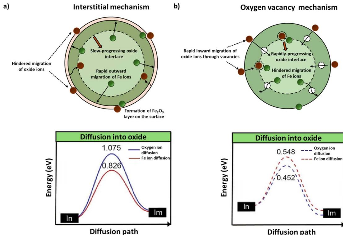
Fig. 3 Ionic diffusion and corresponding activation energy diagram for  $\text{Fe}_2\text{O}_3$  OC under (a) interstitial mechanism. (b) Vacancy mechanism. Green and white spheres indicate Fe ions and oxide ions, respectively, while white spheres depict oxygen vacancies. Energy diagrams adapted from a 2018 article published by Elsevier (ref. 57) under a CC BY-NC-ND 4.0 License.
