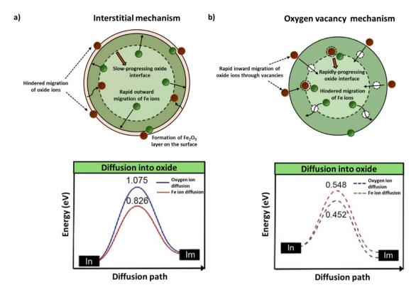
Fig. 3 Ionic diffusion and corresponding activation energy diagram for Fe<sub>2</sub>O<sub>3</sub> OC under (a) interstitial mechanism. (b) Vacancy mechanism. Green and white spheres indicate Fe ions and oxide ions, respectively, while white spheres depict oxygen vacancies. Energy diagrams adapted from a 2018 article published by Elsevier (ref. 57) under a CC BY-NC-ND 4.0 License.
