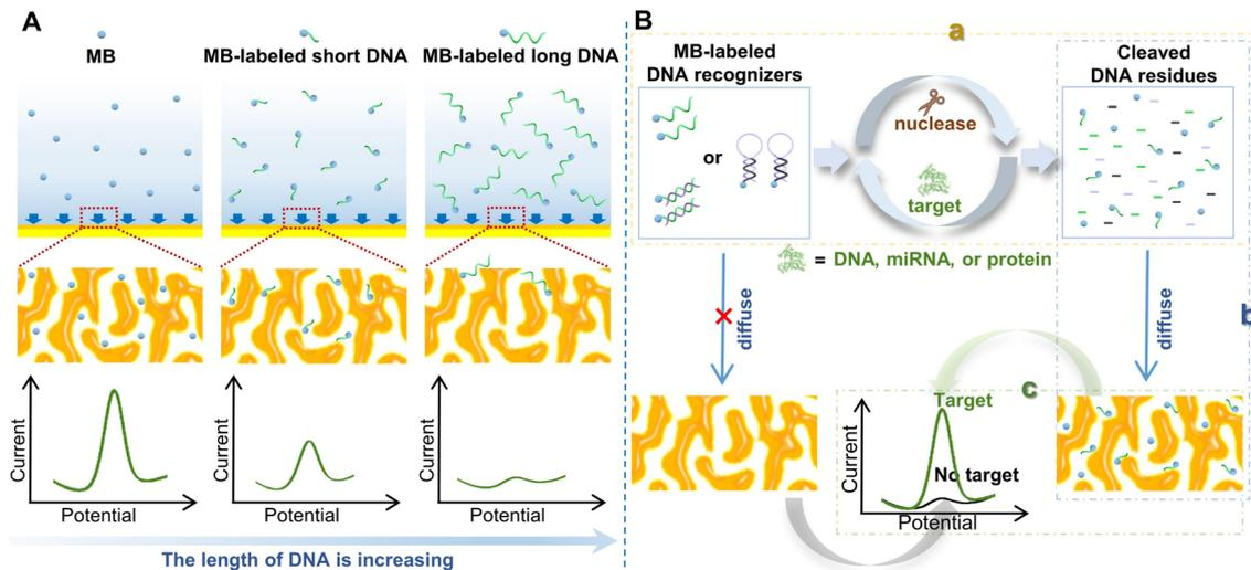
**Scheme 1** (A) Illustration of the response current variation with DNA length on the NPG sensing platform. (B) Schematic diagram of the working principle of the DNA-based NPG electrochemical biosensor for the universal detection of DNA, miRNA, and protein, which is composed of three modules: (a) nuclease-assisted target-recycling recognition and amplification module, (b) NPG platform-based signal molecule enrichment module, and (c) signal conversion module.
