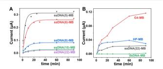
Fig. 1 (A) The DPV response current of NPG/AuE over time in Tris—HCl buffer solution containing 1  $\mu$ M ssDNA(5)-MB, ssDNA(6)-MB, ssDNA(8)-MB, ssDNA(10)-MB, and ssDNA(22)-MB, respectively. (B) The DPV response current of NPG/AuE over time in Tris—HCl buffer solution containing 1  $\mu$ M DNA with different configurations, ssDNA(22)-MB, G4-MB, HP-MB, and dsDNA-MB.
