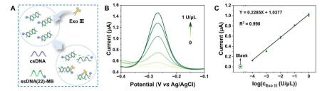
Fig. 2 (A) Schematic diagram of the sensitive detection of Exo III. (B) The DPV response of the NPG/AuE sensing platform towards different concentrations of Exo III (0, 0.0001, 0.001, 0.01, 0.01, and 1 U  $\mu$ L<sup>-1</sup>, respectively). (C) The corresponding linear relationship between response current and the logarithm of Exo III concentration.
