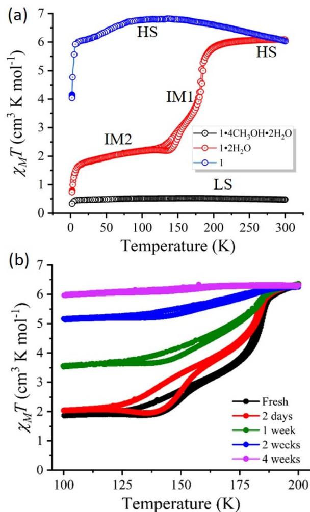
Fig. 3 (a)  $\chi_{\text{M}}T$  vs. temperature plot for complexes  $1 \cdot 4\text{CH}_3\text{OH} \cdot 2\text{H}_2\text{O}$  (black circles),  $1 \cdot 2\text{H}_2\text{O}$  (red circles) and **1** (blue circles) @  $5 \text{ K min}^{-1}$  and (b) the magnetic data of the complex  $1 \cdot 2\text{H}_2\text{O}$  with the ageing of the sample. The magnetic data were measured on the amorphous sample obtained from direct mixing.
