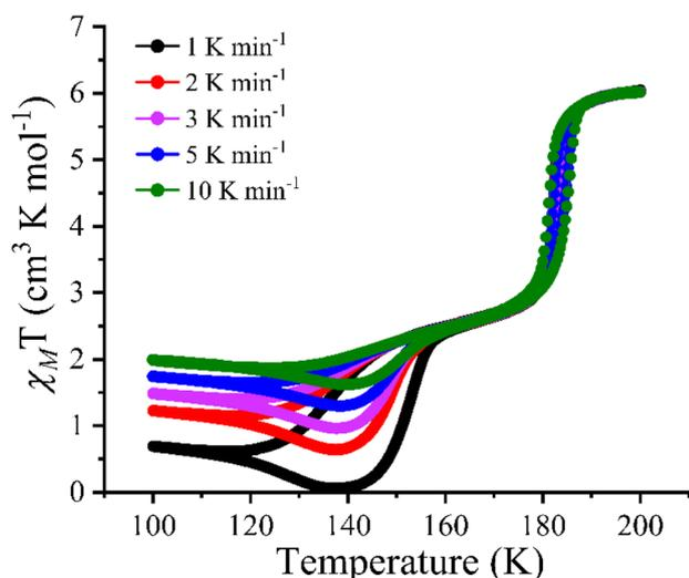
Fig. 5  $\chi_M T$  vs. temperature plot for complex **1**·2H<sub>2</sub>O at different scan rates from 1 to 10 K min<sup>-1</sup> at a 1 T applied magnetic field, showing complete conversion to the diamagnetic state achieved at 140 K. The measurement was performed on the freshly obtained crystals of the complex.
